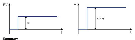
The P controller has the following characteristics:
