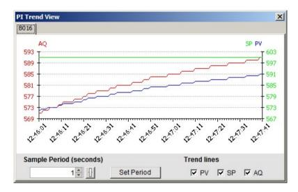
If your circuit program has more than one PI controller function block, the trend view has a separate tab for each PI controller.
