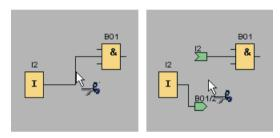
The connection is closed again by clicking on its open end while the Cut/Join tool is active. Optionally, you can close the connection by right-clicking on an open end and calling the **Join** menu command.
