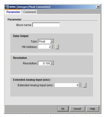
**Data Output**: The output of Integer/Float is stored in VM. You can chose the output type as float or double and the start VM address where the converted float stores.
