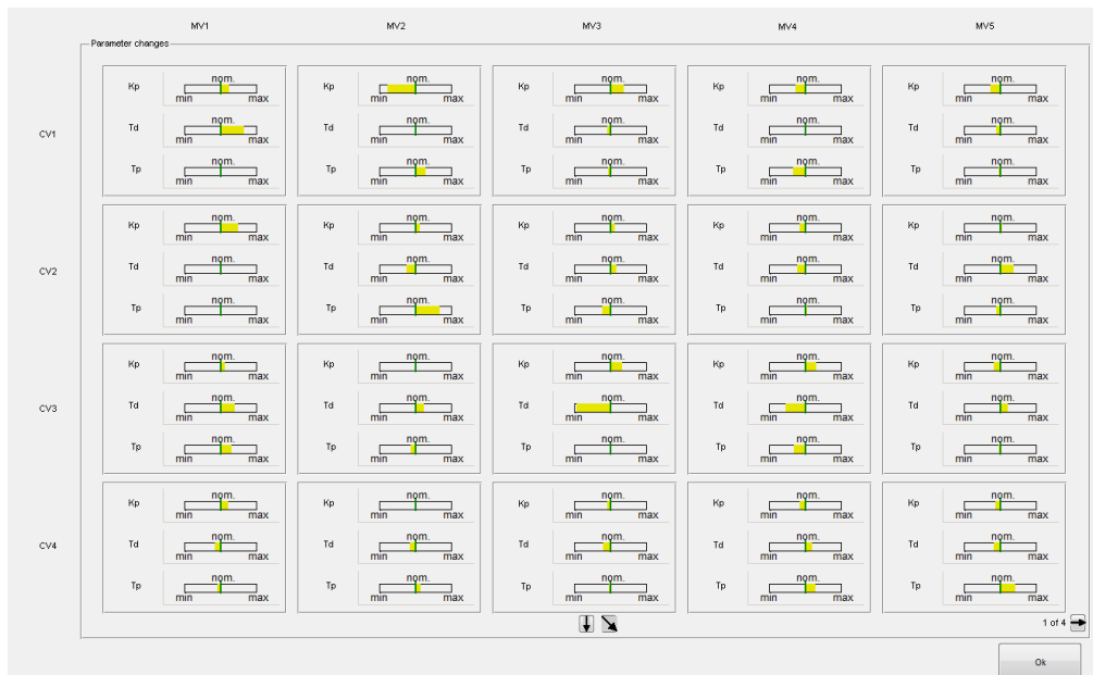
Figure 4-11: Model variations of part transfer functions, in each case K_p : gain, T_d : Dead time and T_p : time constant. The nominal values are represented by the green line, the yellow bar shows the model variation as deviations from nominal value in the range of model accuracy estimated from learning data.
