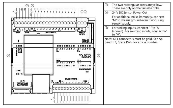
Table A- 41 Connector pin locations for CPU 1214FC DC/DC/DC (6ES7214-1AF40-0XB0)
