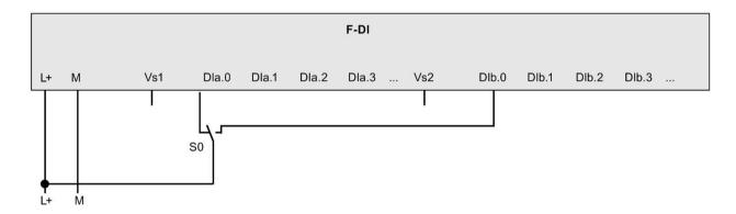
Figure 3-8 F-DI Application mode 8: External sensor supply
