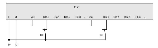
Figure 3-2 F-DI Application mode 2: External sensor supply
