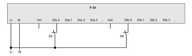
Figure 3-6 F-DI Application mode 6: External sensor supply
