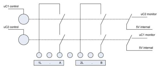
Output channel a.0: Two circuits controlled as one process output channel.
