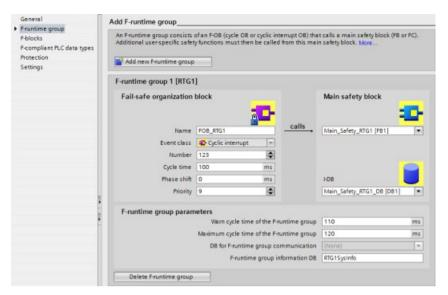
The cyclic interrupt OB (FOB\_1 [OB123]) calls the main safety block (Main\_Safety [FB1]) by default. The F-blocks created by the user are called from the main safety block. You can change the calling block and the called block at any time.
