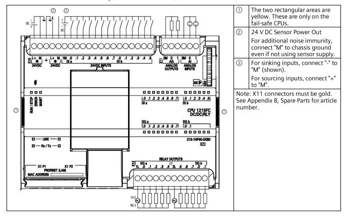
Table A- 58 Connector pin locations for CPU 1215FC DC/DC/Relay (6ES7215-1HF40-0XB0)
