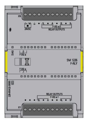
The SM 1226 F-DQ 2 x Relay is an S7-1200 signal module (SM) for use in fail-safe applications. The F-RLY has two output channels (F-DQ a.0 and F-DQ a.1). Each channel includes two circuits that switch mechanically-linked contacts at the same time. Each circuit has two contacts in series controlled by independent relay coils.
