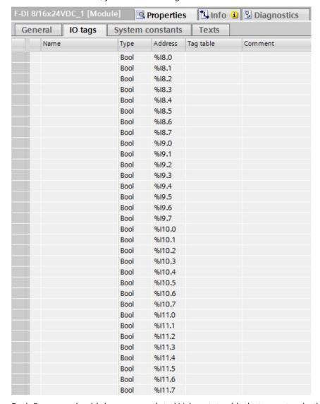
Each Process value bit has an associated Value status bit that reports whether the corresponding process value is valid or passivated. Value status bits are ON for valid data and OFF for data associated with passivated channels. If an entire module or a single channel is passivated, the associated Value status bits are OFF.
