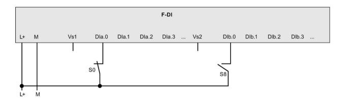
Figure 3-10 F-DI Application mode 10: External sensor supply
