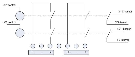
Output channel a.0: Two circuits controlled as one process output channel Refer to the isolation description in the SM 1226 F-DQ 2 x Relay (Page 190) specifications, Digital outputs table.
