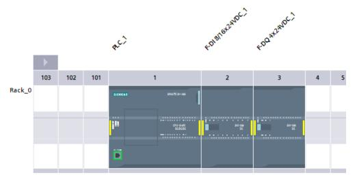
2. Open "Device data" to display the "Device overview" area. Here, you can change the start addresses for the inputs and outputs of your fail-safe module. Use the module default I/O addresses of "17" and "17" for this example (inputs begin at byte 17, and outputs begin at byte 17).
