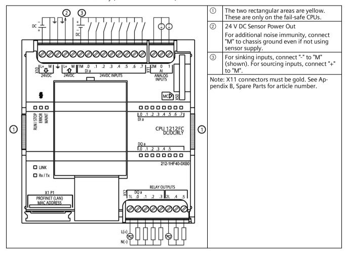
Table A- 22 Connector pin locations for CPU 1212FC DC/DC/Relay (6ES7212-1HF40-0XB0)
