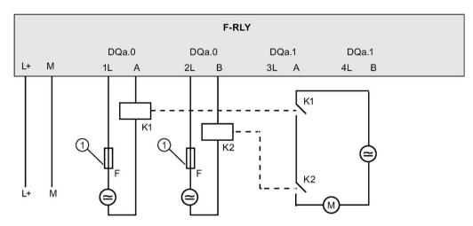
① External fuse (Refer to F-DQ 2 x Relay "Specifications" (Page 190), "Digital outputs" table, "Short-circuit protection of output" for external fuse details.)
