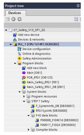
The first step in programming of the safety program is the main safety block. The main safety block is an F-FB (with instance DB) that is called from the "Fail-Safe Organization Block" (F-OB) (cyclic interrupt OB) assigned in each F-runtime group. The F-OB has a higher priority than other standard OBs.
