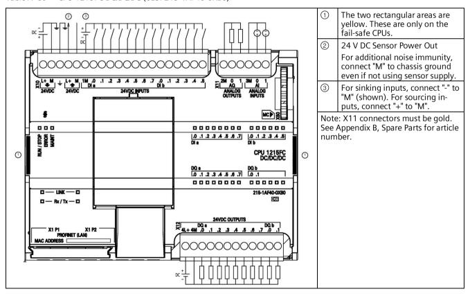
Table A- 60 Connector pin locations for CPU 1215FC DC/DC/DC (6ES7215-1AF40-0XB0)
