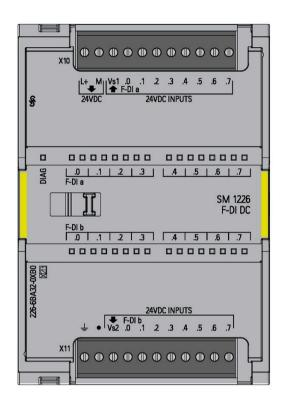
The SM 1226 F-DI 16 x 24 V DC is an S7-1200 signal module (SM) for use in fail-safe applications. The inputs are rated for connection to 24 V DC sensors/switches and 3/4-wire proximity switches (for example, BEROs: Siemens line of no-touch sensors) and have an EN61131-2 type 1 input rating.
