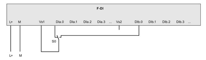
Figure 3-7 F-DI Application mode 7: Internal sensor supply
