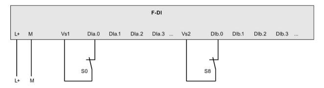
If short circuit detection is used, VS1 must be used with a.x inputs and VS2 must be used with b.x inputs.
