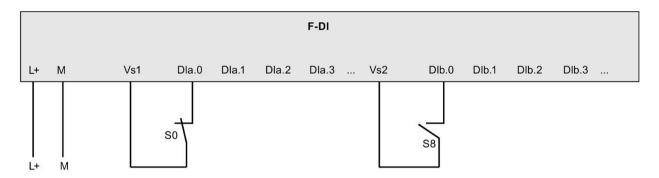
Figure 3-9 F-DI Application mode 9: Internal sensor supply
