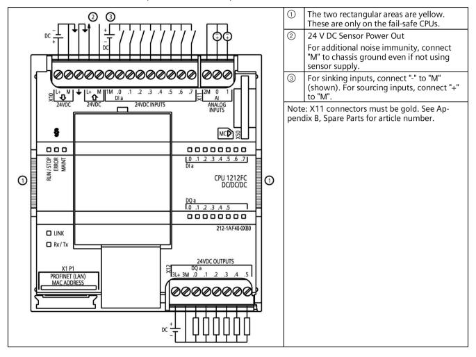
Table A- 24 Connector pin locations for CPU 1212FC DC/DC/DC (6ES7212-1AF40-0XB0)
