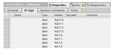
Each Process value bit has an associated Value status bit that reports whether the corresponding process value is good. Value status bits are ON for good quality and OFF for bad quality. If an entire module or channel is passivated, the associated Value status bits are OFF.
