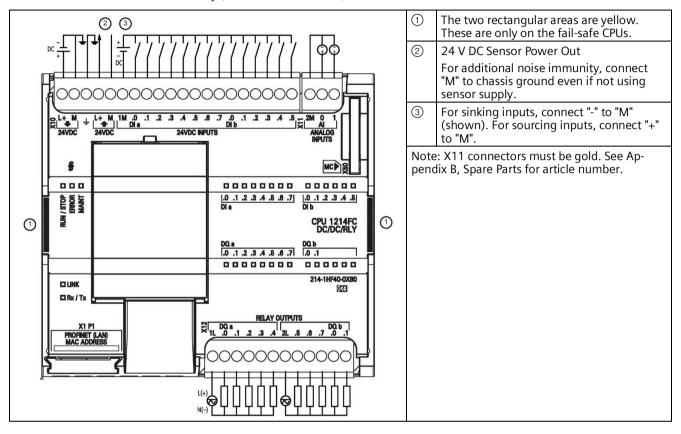
Table A- 39 Connector pin locations for CPU 1214FC DC/DC/Relay (6ES7214-1HF40-0XB0)
