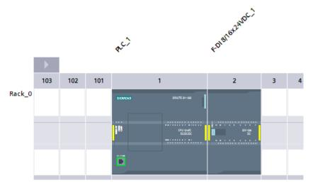
2. Open "Device data" to display the "Device overview" area. Here, you can change the starting addresses for the inputs and outputs of your fail-safe module. Use the module default I/O addresses of "8" and "8" for this example (inputs begin at byte 8, and outputs begin at byte 8).
