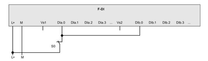
Figure 3-4 F-DI Application mode 4: External sensor supply
