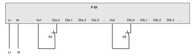
Figure 3-5 F-DI Application mode 5: Internal sensor supply
