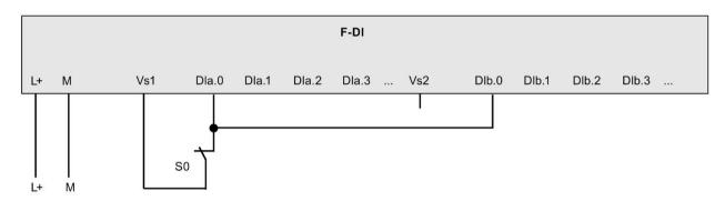
Figure 3-3 F-DI Application mode 3: Internal sensor supply
