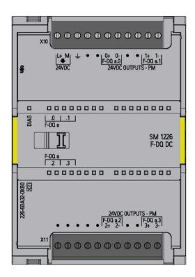
The SM 1226 F-DQ 4 x 24 V DC is an S7-1200 signal module (SM) for use in fail-safe applications and is suitable for solenoid valves, DC contactors, and indicator LEDs. It has four outputs with P- and M-switching that are rated for connection to 24 V DC actuators with up to a 2.0 A rating.
