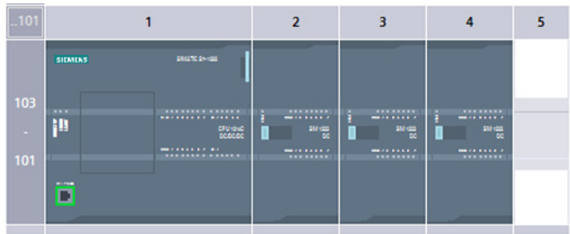
Figure 6-1 Device configuration of maximum installation
