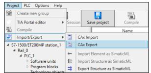
Device data are exported in AML format with the CAx export. The CAx export is possible on the project level or on the device level.
