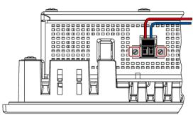
Secure the connection terminal with the marked screws.
