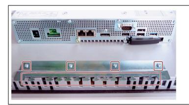
Secure the connecting cables with cable ties at a suitable point in the marked area.
