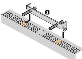
Secure the mounting bracket by tightening the threaded pins. The maximum permissible torque is 0.5 Nm.
