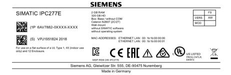
The Ethernet addresses can also be found in the BIOS Setup under "Main > Advanced > Peripheral Configuration" (see section "Technical Specifications").
