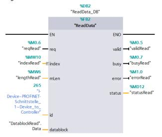
**Note** Use the HW identifier stored in the system constants for the input "id". If a transfer area was created, its HW identifier will be stored in the system constants and can be used symbolically.
