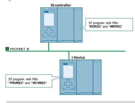
**Note** The function blocks "RDREC", "WRREC", "PRVREC" and "RCVREC" are located in the "Extended Instructions" of the TIA portal.
