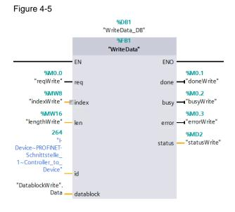
**Note** Use the HW identifier stored in the system constants for the input "id". If a transfer area was created, its HW identifier will be stored in the system constants and can be used symbolically.
