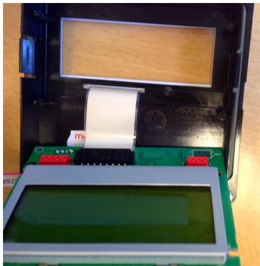
6. Repeat these steps in reverse order to connect the replacement unit. Ensure that connection band to user interface is connected correctly.
