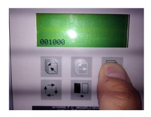
Press the key again. The transmitter will continue powering up and then enter measuring mode.
