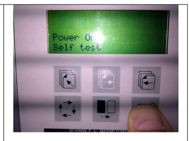
Then press the key again. All pixels in display will start flashing. If all pixels within all characters can are toggled on / off, the display is OK.
