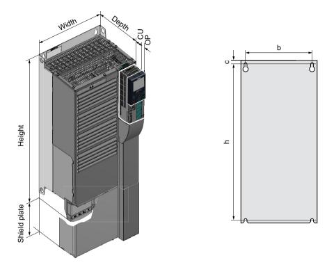
Table 4-3Dimensions depend on the Control Unit (CU) and Operator Panel (OP)
