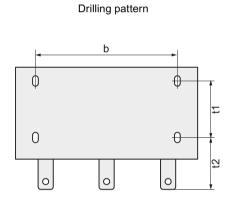
Figure 8-7 Standalone output reactor for frame sizes FSD ... FSF
