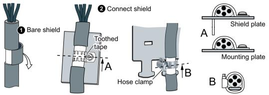
Figure 4-3 Examples for EMC-compliant shield support
