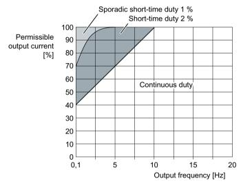
Figure 7-1 Permissible operating range of the converter
