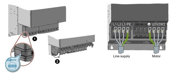
You must open the cover to connect the line and motor:
