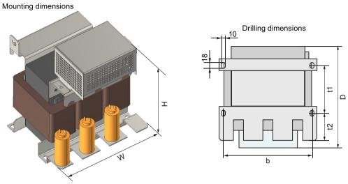
Figure 8-10 Dimensions - standalone filter
