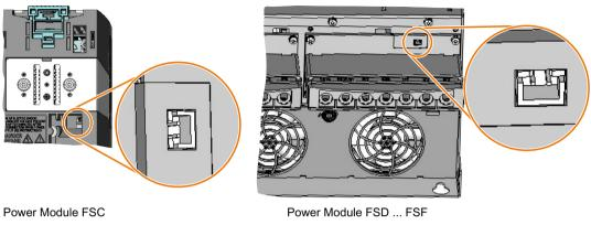
Figure 8-12 Connector position for the Brake Relay
