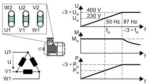
In a delta connection, the motor is operated with a voltage and frequency above its rated values. As a consequence, the motor power is increased by a factor  $\sqrt{3} \approx 1.73$ .
