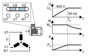
In a star connection, the motor can provide its rated torque  $M_N$  in the range 0 ... rated frequency  $f_N$ .
