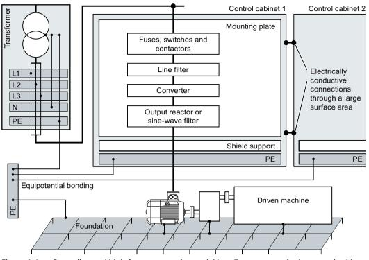
Figure 4-4 Grounding and high-frequency equipotential bonding measures in the control cabinet and in the plant/system
