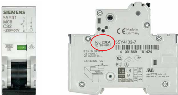
Figure 11a: MCB labeling example, approved in accordance with IEC/EN 60898-1, additional labeling Icu in accordance with IEC/EN 60947-2
