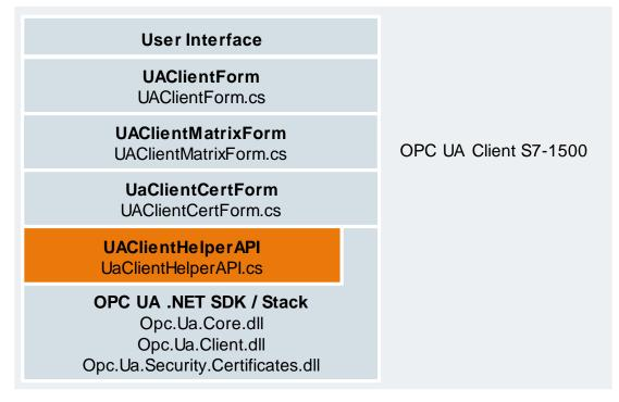
The "UAClientForm" class is derived from the Windows.Forms system class and includes the form constructor as well as the EventHandlers of the program interface. The methods of the "UAClientHelperAPI" class are accessed in the EventHandlers.
