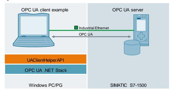
A simple OPC UA .NET client for Windows PCs/PGs communicates with the OPC UA server of a SIMATIC S7-1500.
