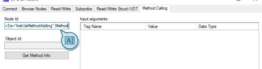
5. Click the "Get Method Info" button to receive the object id and the input and output arguments of the method.
