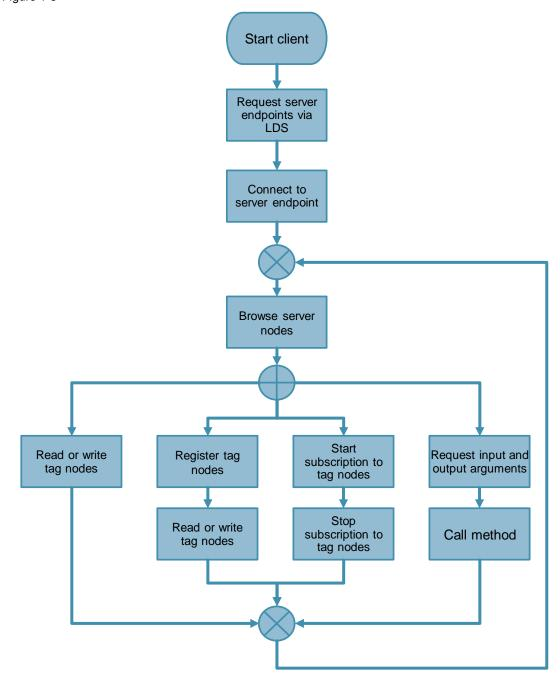
**NOTE** In order to request server endpoints via a LDS (Local Discovery Server) or GDS (Global Discovery Server) a LDS has to be installed on the PC/PG or a GDS has to be available in the network.
