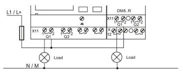
Protection with automatic circuit-breaker, max. 16 A, characteristics B16, e. g.: Power circuit-breaker 5SX2 116-6 (if required)
