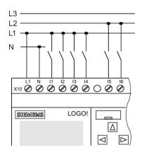
The inputs of these devices are in two groups, each consisting of four inputs. Different phases are only possible between blocks, but not within the blocks.
