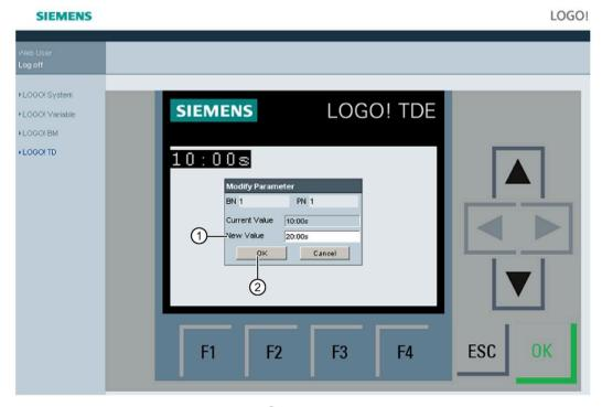
Enter the desired parameter value in line "①" on the above screens. In this example, enter "20:00s".
