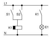
You already know the first part of the circuit. S1 and S2 switch a relay, which is to be used to switch on the load E1, and to switch off the load with a delay of 12 minutes.
