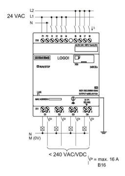
The inputs of these devices are not isolated and therefore require a common reference potential (chassis ground).
