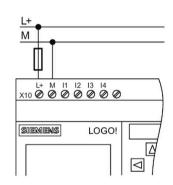
Protection with safety fuse if required (recommended) for: 12/24 RC...: 0.8 A 24: 2.0 A
