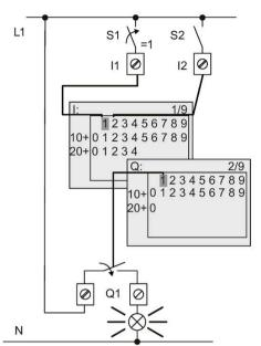
When switch S1 is closed, the status at input I1 is high.
