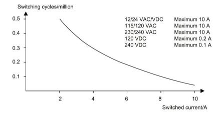
Switching capacity and service life of the contacts with high inductive load to IEC 60947-5-1 DC 13/AC 15 (contactors, solenoid coils, motors):
