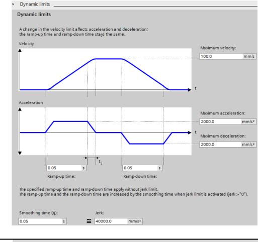
**CAUTION** If the motion of at least one axis is limited, this may cause a deviation of the desired trajectory. This is why you should make sure that the limitations of the traversing axes are not reached during the interpolated motion.
