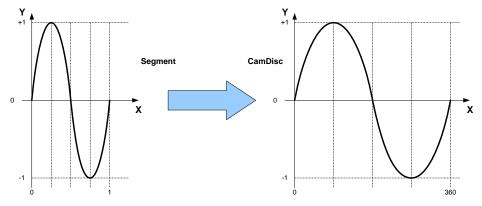
Figure 3-6: Example for the transformation of the segment in the curve disc
