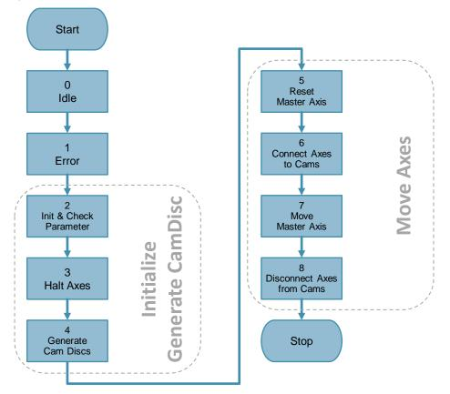
Circular Motion on the Basis of Cam Discs "MoveCircle2D" Entry-ID: 109742306, V1.1, 04/2017 The individual steps of the block have the following function:
