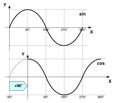
The curves for sinus and cosinus each have to be standardized for the range  $0 \le X \le 1$  in the trigonometric fraction of the segment. The function value of the two angle functions have to be in the range of  $-1 \le Y \le +1$ . Thus the following assignment results for the two missing parameters of the angle functions:
