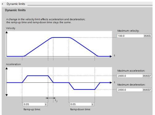
The specified ramp-up time and ramp-down time apply without jerk limit. The ramp-up time and the ramp-down time are increased by the smoothing time when jerk limit is activated (jerk > "0").
