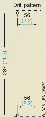
Fixing with M4 bolts
