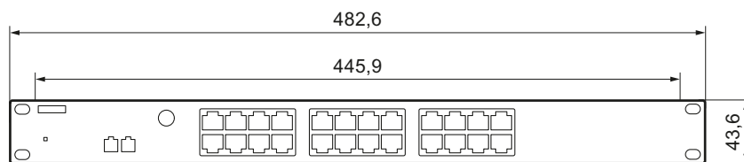
Figure 7-1 Width and height based on the example of a 24 V DC variant
