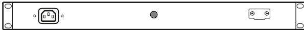
Figure 4-5 Position of the grounding bolt on the back of the device for PoE variants.
