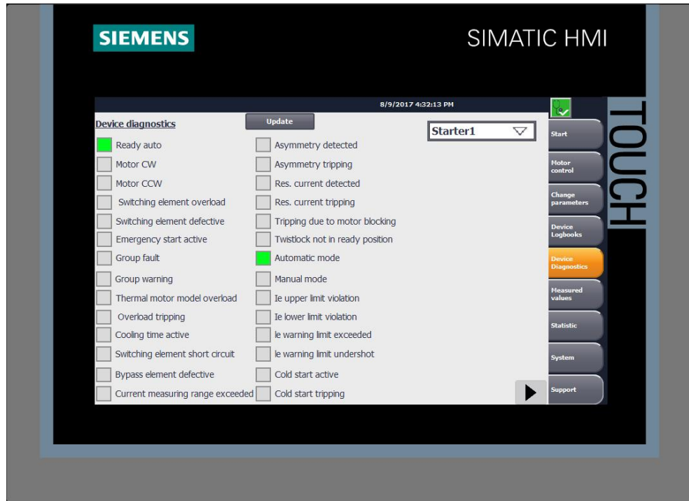
Figure -4-15 HMI screen “Device diagnostics” 1
