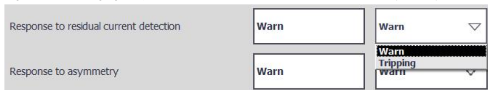
Figure 4-10 Changing the parameters “Residual current detection” and “Asymmetry”
