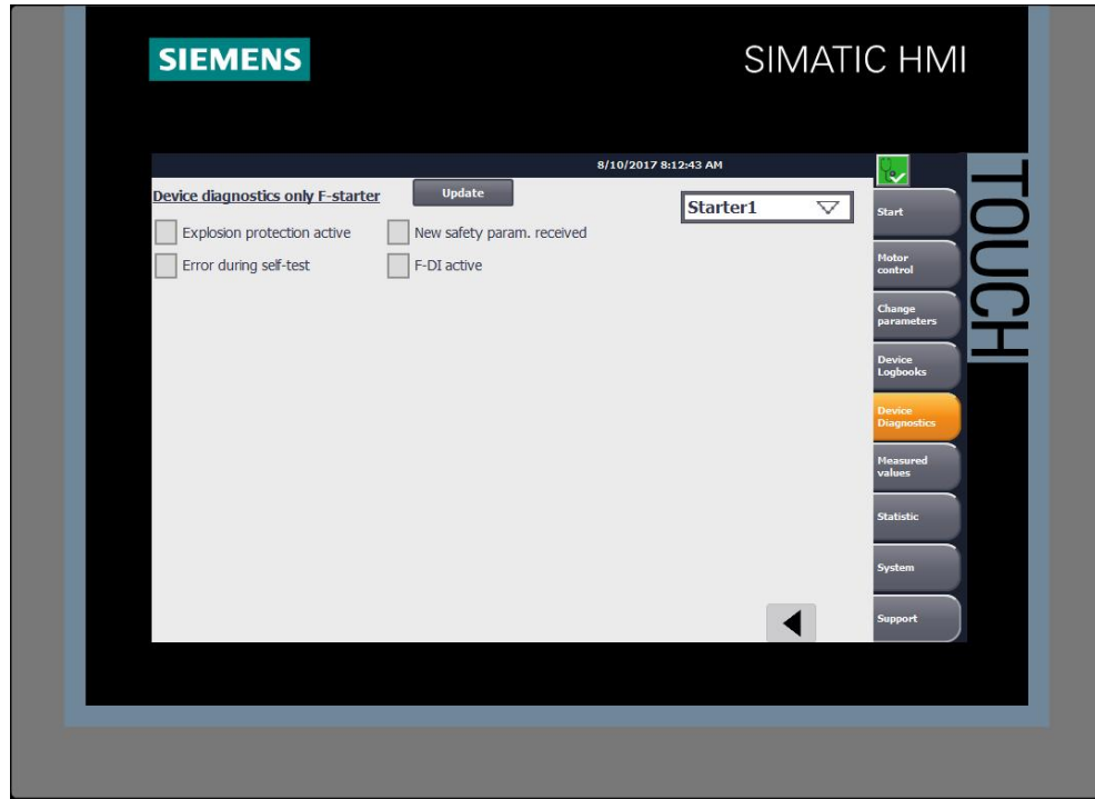
Figure -4-18 HMI screen “Device diagnostics F-motor starter”
