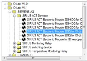
Select "SIRIUS ACT electronics module for ID key switches" from the catalog under "IO Link v1.1 > SIEMENS AG > SIRIUS ACT devices" and move it to port 2 in the normal working range.
