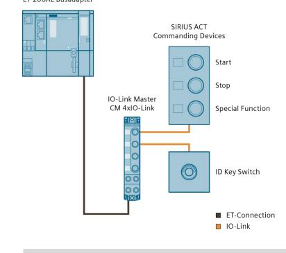
**Note** Take note that the distance between the bus adapter and the IO-Link master must not exceed a maximum 15 m since this corresponds to the maximal possible bus line length for the ET-connection.
