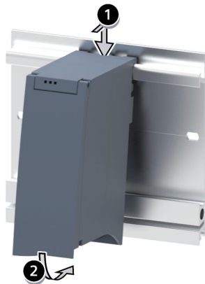
Figure 7-10 Installing a load current supply
