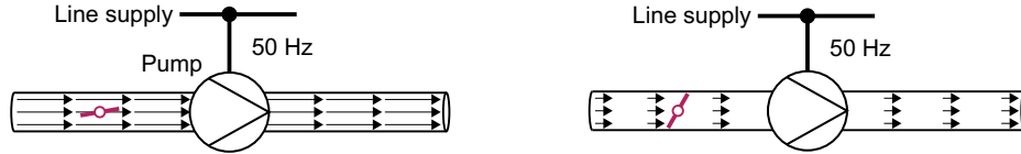
Figure 6-82 Flow control with pump and throttle connected to a 50 Hz line supply
