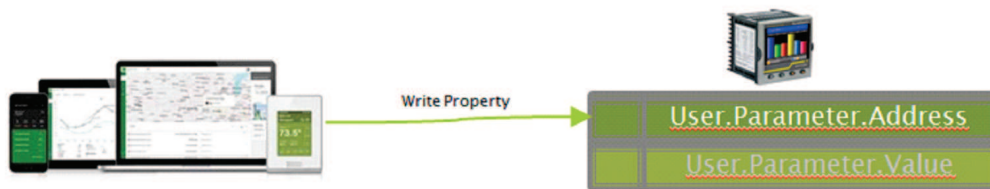
Figure 109 BMS Client writes address of required parameter
