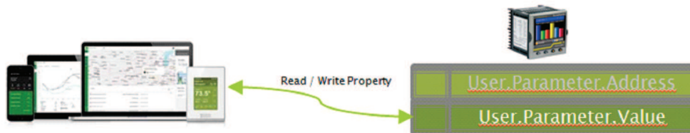
Figure 110 BMS Client reads/writes to data parameter
