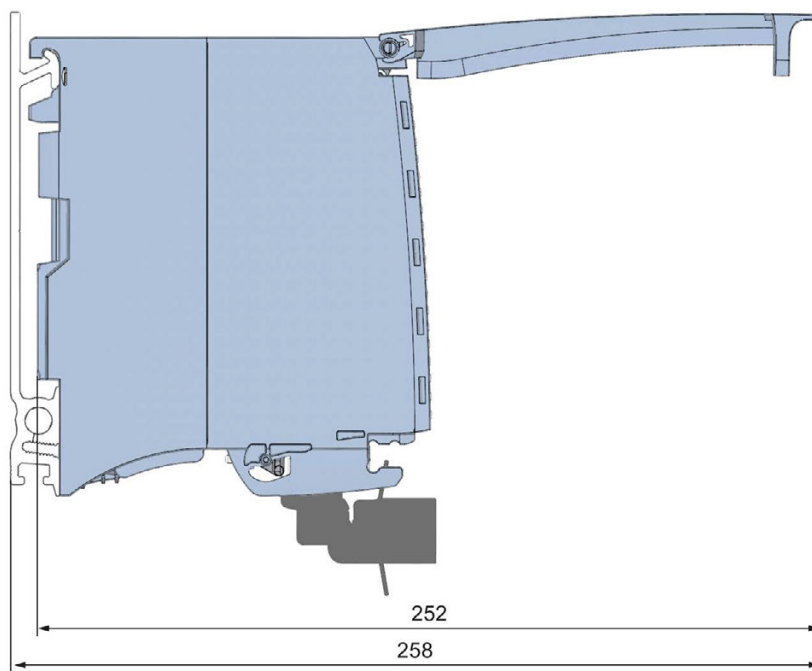
Figure A-2 Dimension drawing of the AI 8xU/I/R/RTD BA module, side view with open front cover
