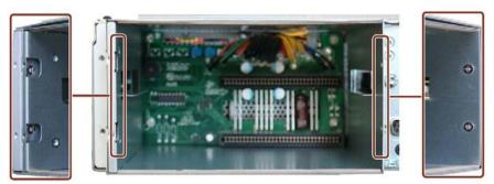
2. Loosen the screws marked in the following picture at the enclosure bottom.
