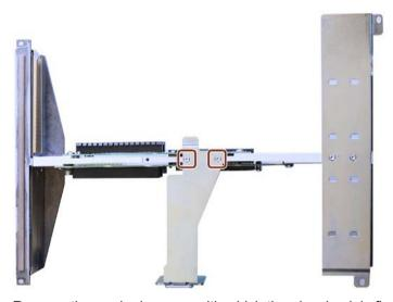
2. Remove the marked screws with which the piggyback is fixed to the center rail.
