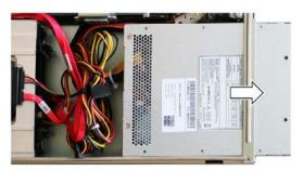
4. Remove the cable ties securing the power cables in the enclosure.
