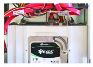
5. Press both clips inward at the same time; the drive automatically slides out.
