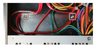
4. Remove the screws marked in the following picture.
