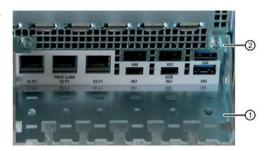
Insert the detachable cable ties in the respective openings of the strain relief and fasten the cables with the cable ties.
