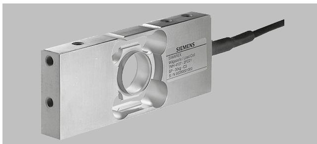
The SIWAREX WL260 SP-S SB platform load cell is excellently suited for use in platform scales with dimensions up to and including 350 x 350 mm (13.78 x 13.78 inch). It is approved for use in Class III weighing machines with maximum divisions of  $n_{\max}$  to 3 000d.
