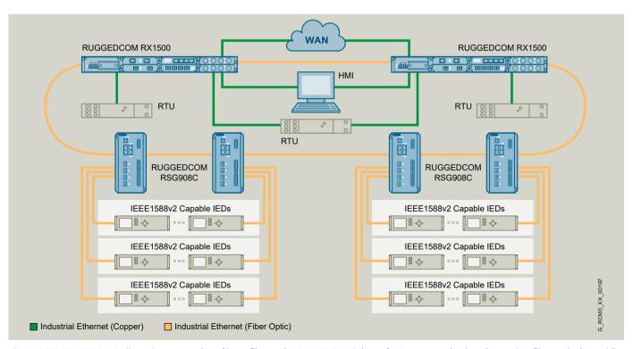
The RUGGEDCOM RSG908C allows the aggregation of large fiber optic 100BASE-FX subrings of IEDs at protection bays into 1 Gbps fiber optic rings while providing IEEE 1588 timing.
