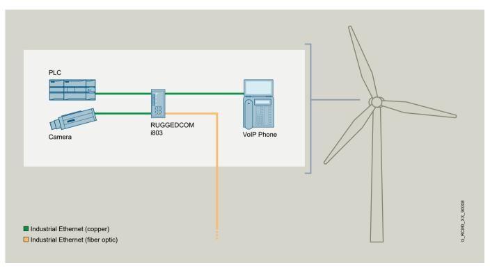
Inside the nacelle of a wind turbine, the RUGGEDCOM i802 enables connectivity for up to 6 Ethernet devices over copper and a backhaul over fiber-optic.
