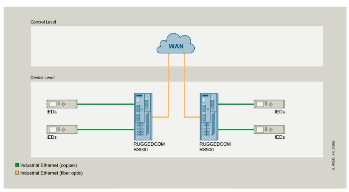
The RUGGEDCOM RS900 makes it possible to remotely monitor field data using multiple types of communications.
