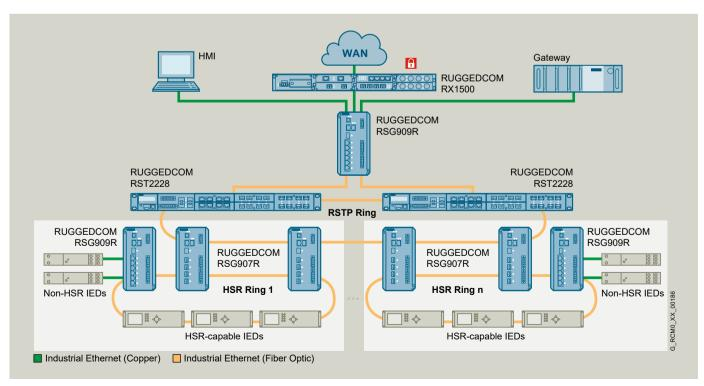
RUGGEDCOM RSG907R/RSG909R switches terminating each HSR ring can be directly connected to an RSTP network via their coupling ports.
