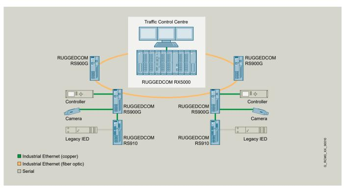
A reliable eRSTP ring network with Gigabit bandwidths can be achieved with the RUGGEDCOM RS900G.
