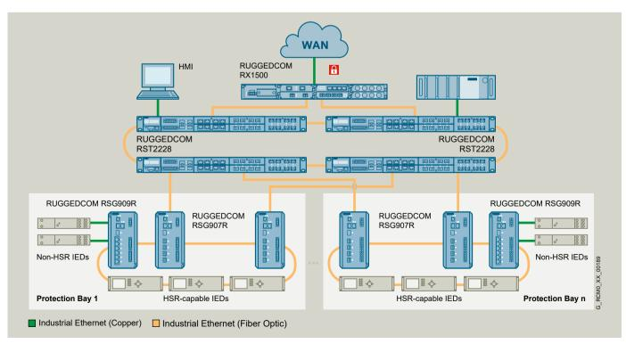
Two RUGGEDCOM RSG907R/RSG909R are used in each HSR bay ring for redundant coupling with PRP station level LANs.
