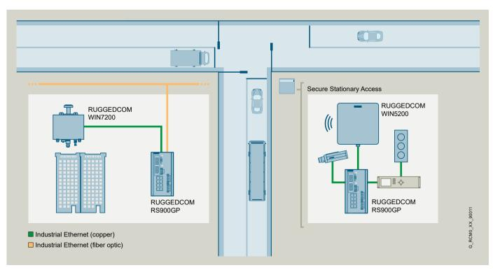
Multiple Power-over-Ethernet devices are powered by the RUGGEDCOM RS900GP in the field.
