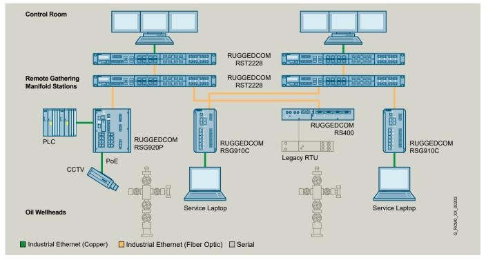
Wellhead monitoring in onshore oil and gas production with the RUGGEDCOM RSG910C
