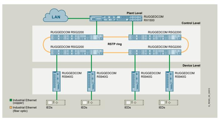
The RUGGEDCOM RS940G can connect up to 8 devices with Gigabit speeds on the device level.
