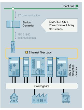
The PC-based station controller unites the functions of a PCS 7 automation system with the integration of protection devices at a highly favorable price/performance ratio
