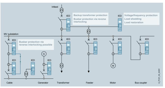
Basic structure of typical medium-voltage switchgear
