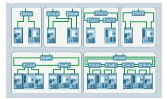
Typical examples of the integration of protection devices in a complete configuration using different network topologies
