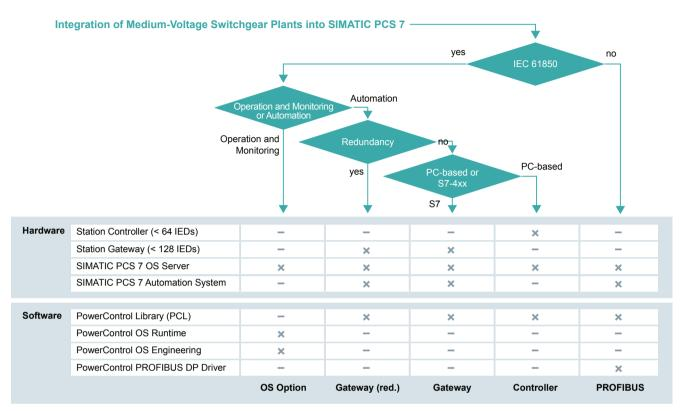
Selection aid with various possibilities for integration of switchgears in SIMATIC PCS 7
