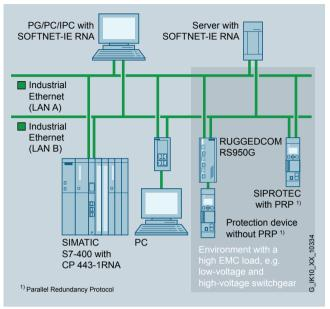
Example configuration: redundant network topology with PRP communication
