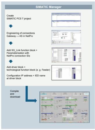
Workflow for engineering of PCS 7 PowerControl with station gateway (symbols and faceplates generated in corresponding OS picture)
