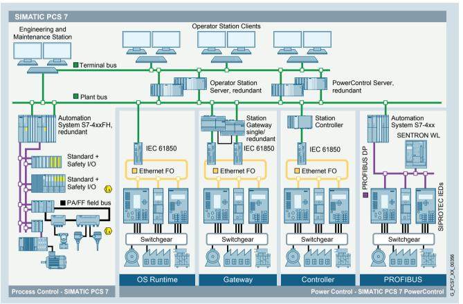
Merging of process control system and station control system. There are several ways to achieve integration: Directly on the plant bus, via station gateway, via station controller, or via PROFIBUS DP.
