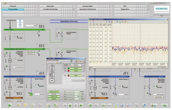
Example of a plant display for medium-voltage switchgear with trend window and a faceplate for a medium-voltage motor
