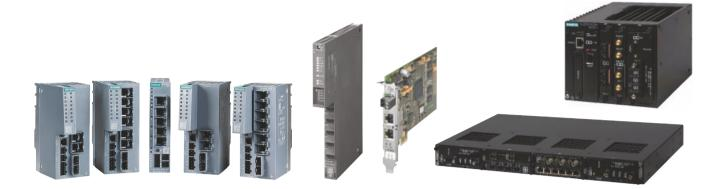
Devices with "Security Integrated": Industrial Security Appliances SCALANCE S, Security CP 443-1 Advanced for S7-400 or CP 1628 for PCs and RUGGEDCOM RX1500 or RX1511
