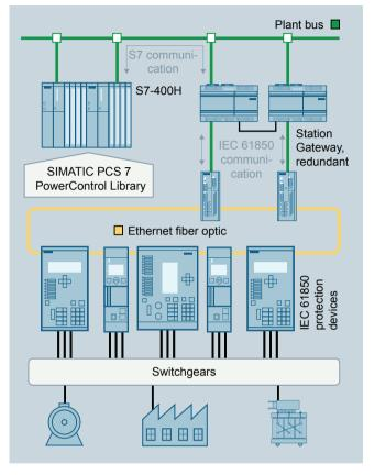
A redundant station gateway supports a larger number of protection devices and provides increased availability
