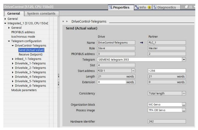
Figure 9-38 Configuring telegrams as isochronous
