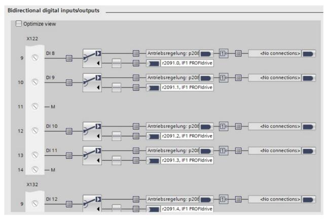
Figure 9-31 Bidirectional inputs/outputs
