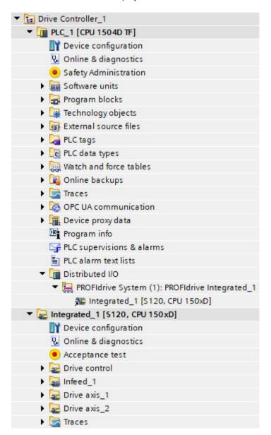
**Under the "Drive Controller" group folder**, you will find both the CPU and SINAMICS Integrated.
