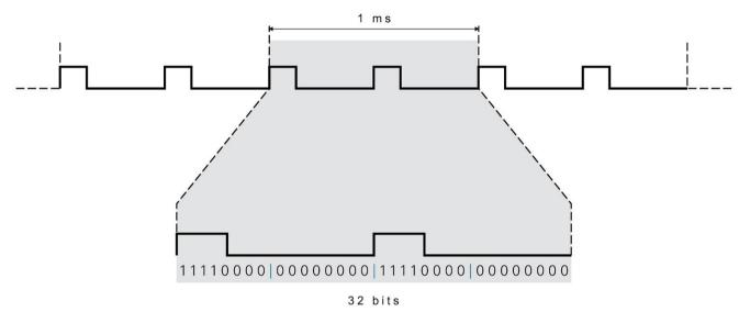
Figure 9-28 Pulse width modulation
