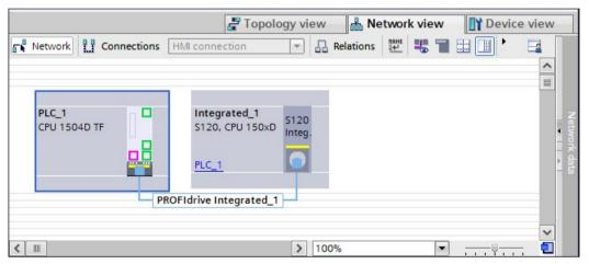
Figure 9-33 SIMATIC Drive Controller in the network view
