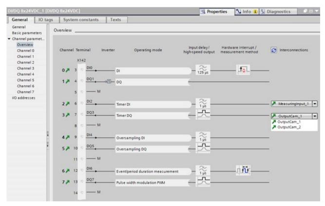
Figure 9-10 Channel parameters
