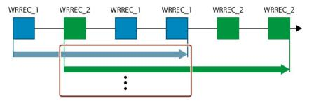
Figure 10-2 Parallel processing of the asynchronous instruction WRREC
