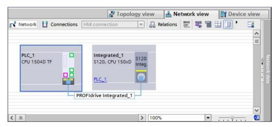
Figure 9-2 SIMATIC Drive Controller network view
