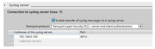
Figure 4-3 Transfer of syslog messages to a syslog server configured
