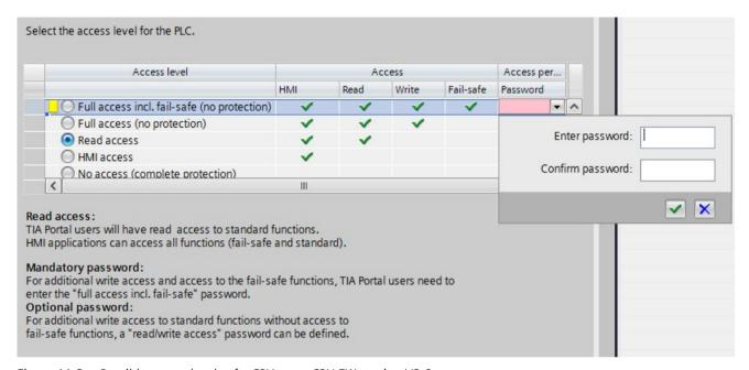
Figure 11-3 Possible access levels of a CPU up to CPU FW version V3.0
