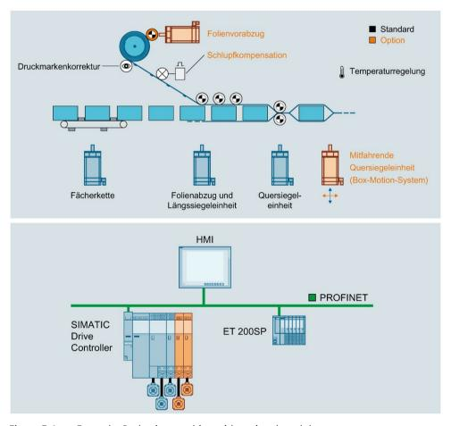
Figure 5-1 Example: Packaging machine with optional modules
