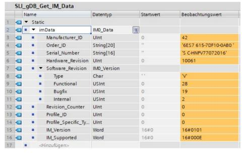
Figure 13-6 Example: I&MO data of an S7-1500 CPU
