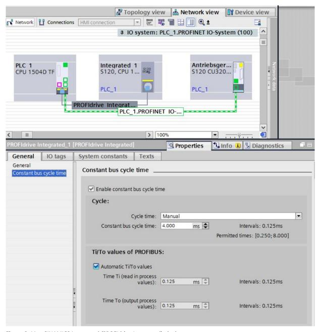
Figure 9-41 SINAMICS Integrated (PROFIdrive Integrated) clock system
