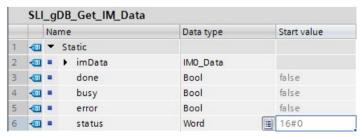
Figure 13-4 Example: Data block for I&M data
