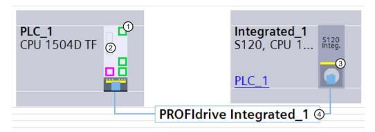
Figure 9-5 Display in the TIA Portal – network view
