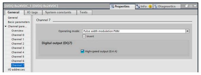
Figure 9-30 Pulse width modulation channel
