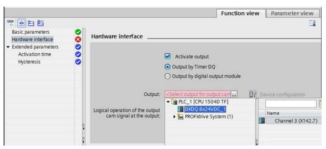
Figure 9-40 Assigning a channel to the output cam
