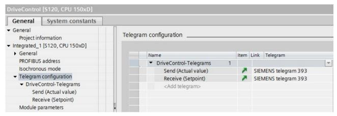
Figure 9-32 Configuration of frame 393 for automatic speed control
