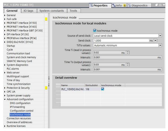
Figure 9-42 Technology I/O clock system
