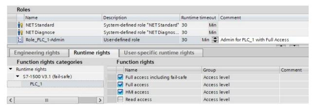
Figure 11-1 Assigning function rights of a CPU to a role
