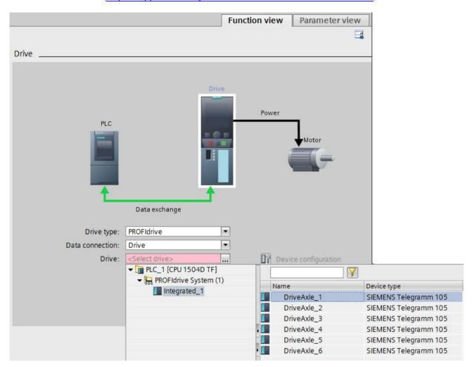
Figure 9-36 Assigning drives to the technology objects
