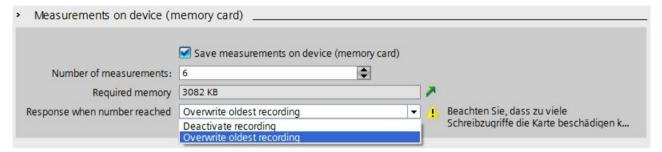
Figure 14-2 Dialog with settings for saving measurements to the memory card in STEP 7
