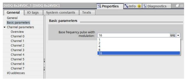
Figure 9-29 Base frequency of pulse width modulation
