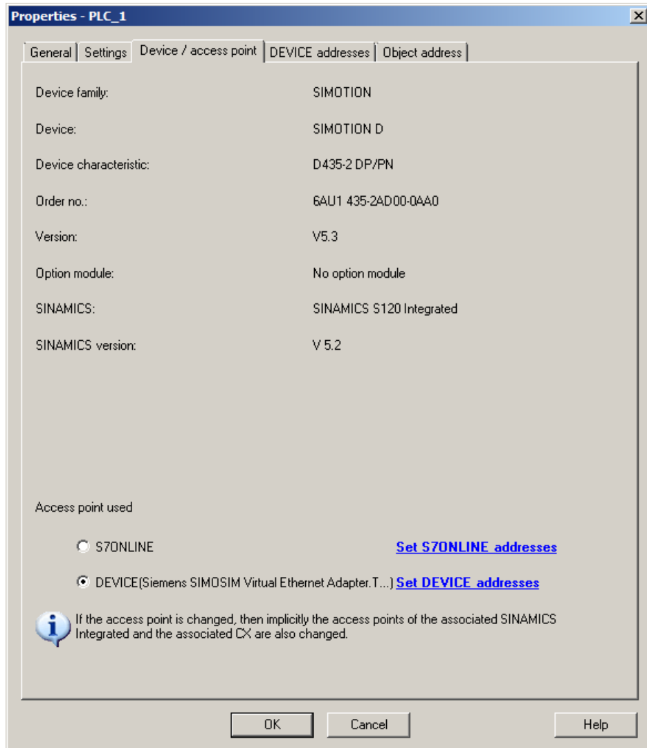
Figure 3-201 Access point used by SIMOSIM
