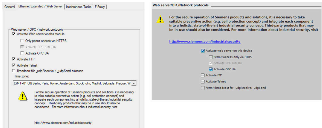
Figure 4-949 Activating the SIMOTION IT Web server functions in SIMOTION SCOUT or SIMOTION SCOUT TIA
