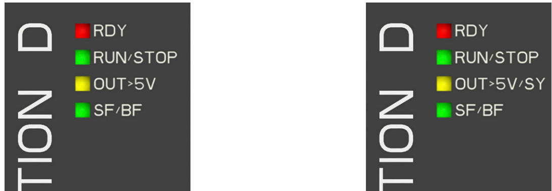
Figure 10-284 LED displays: D410-2 DP (on the left), D410-2 DP/PN (on the right)
