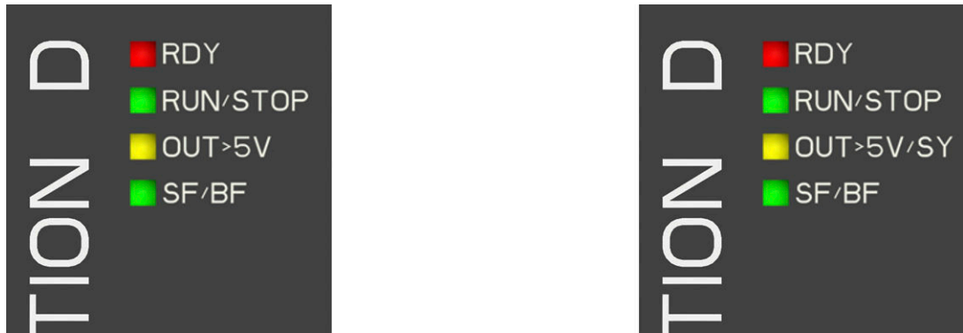
Figure 10-221 LED displays: D410-2 DP (pictured on the left), D410-2 DP/PN (pictured on the right)
