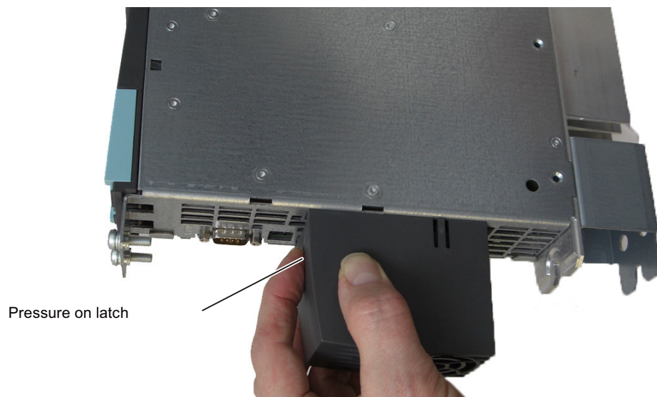
Figure 10-123 Unlatching the fan/battery housing
