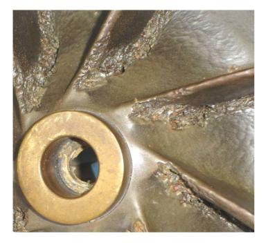
Picture 2: Damage in a Pump by Cavitation
