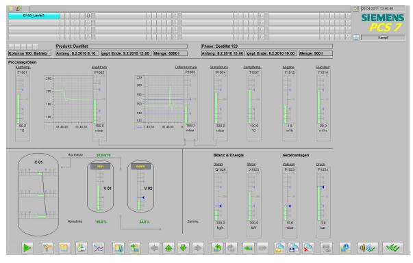
Fig. 2: Overview diagram of the column
