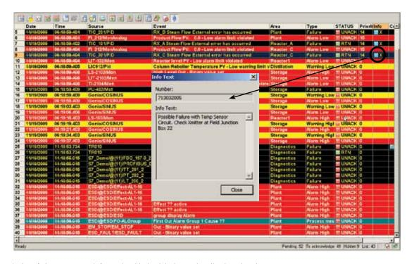
Figure 8 Display of alarm response information (derived during Rationalization phase)
