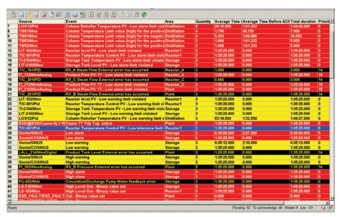
Figure 9 Pinpointing nuisance alarms from an alarm frequency display in the HMI
