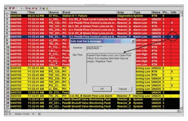
Figure 10 Tools for comparing the online system to the Master Alarm Database
