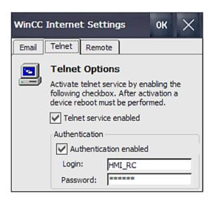
All changes in the "Telnet" tab take effect immediately after clicking "OK"; it is not necessary to restart the HMI device.
