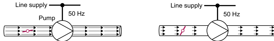
Figure 8-139 Flow control with pump and throttle connected to a 50 Hz line supply
