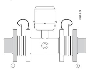
1 Plastic pipes or lined metal pipes
