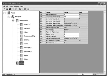
Figure C-5 Battery configuration
