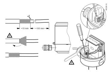
Choose the correct glands for the selected cable type, see Accessories for glands selection. Ensure shield is mounted under cable clamps - do not make pig tails.
