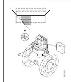
A hardware key is installed in the HL hole to change protected parameters. The HL hole is located in the front of the PCB board behind the battery.
