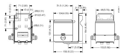
Figure 10-1 Dimensions in mm (inch), weight 3.5 kg (8 lbs)
