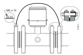
Isolate meter from pipeline by mounting isolation sleeves and washers on flange bolts and connect a wire dimensioned to manage the cathodic current and environmental influence, between pipelines.
