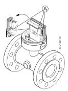
Figure 4-9 MAG 8000 CT verification sealing (A)
