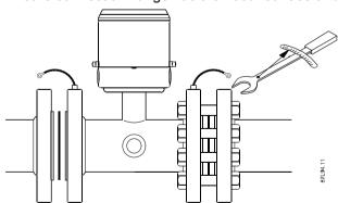
Gaskets are recommended but not included in water meter delivery.
