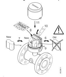
6. Remove battery pack with power still connected.
