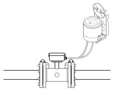
Figure 4-2 Remote installation
