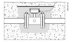
Remote sensor is protected to IP68/NEMA 6P and can be buried.
