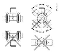
Sensor must be mounted as shown in upper part of figure. Do not mount sensor as shown in lower part of figure as electrodes then will be positioned at top where air bubbles may occur and in bottom, where mud, sludge, sand etc. may deposit and cover the electrode, thus impacting the measurement.
