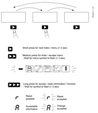
Figure 7-2 Key and display operation
