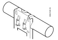
Figure 4-8 Pipe mounting - horizontal
