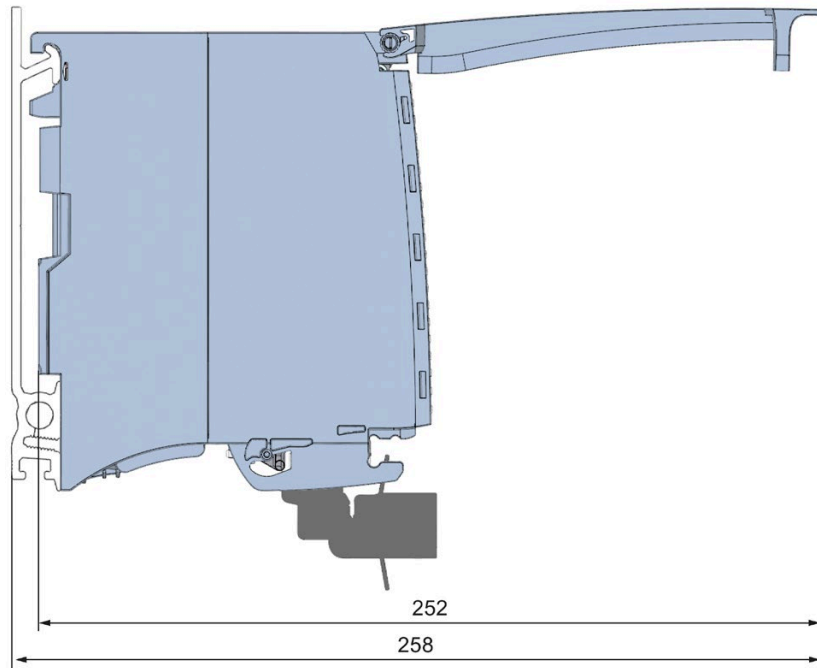
Figure A-2 Dimensional drawing of the AI 16xI BA module, side view with open front cover
