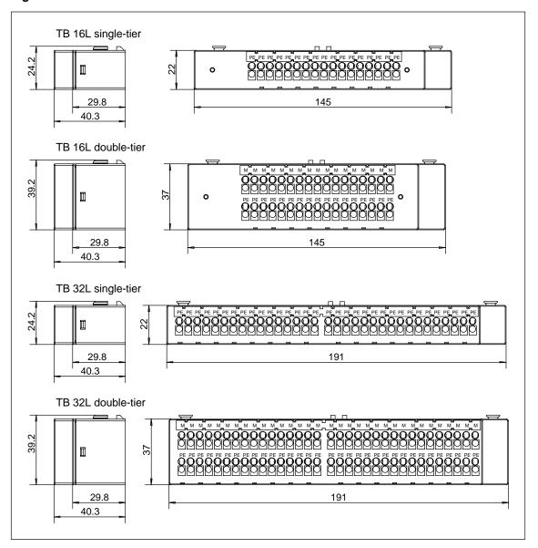
Figure 7-3 TB 16L/TB 32L Supplementary Terminals, Dimension Drawing
