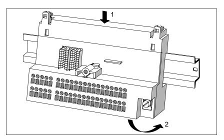
Figure 2-1 Installing the Terminal Block
