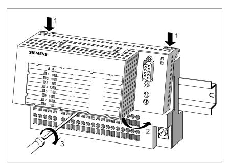
Figure 2-3 Installing the Electronics Block
