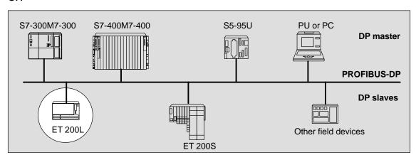
Figure 1-1 A Typical PROFIBUS-DP Installation
