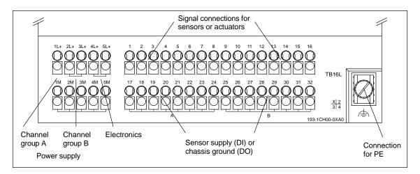
Figure 3-3 Terminal Connections on Terminal Block TB 16L
