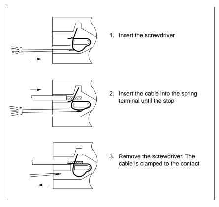
Figure 3-2 How the Spring Terminal Works
