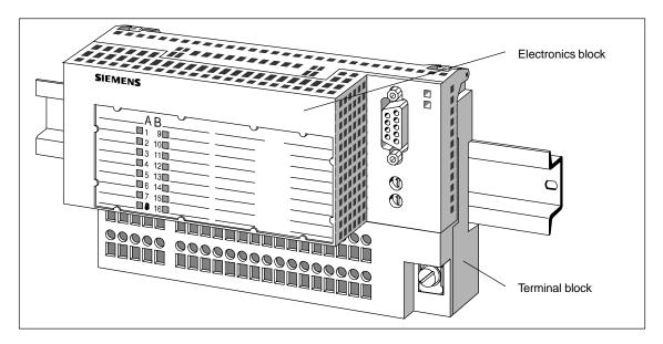
Figure 1-2 View of the ET 200L Distributed I/O Device
