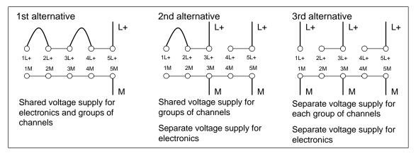
Figure 3-4 Alternative Ways of Connecting the Voltage Supply
