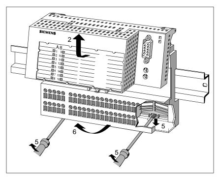
Figure 2-2 Disassembling the Terminal Block
