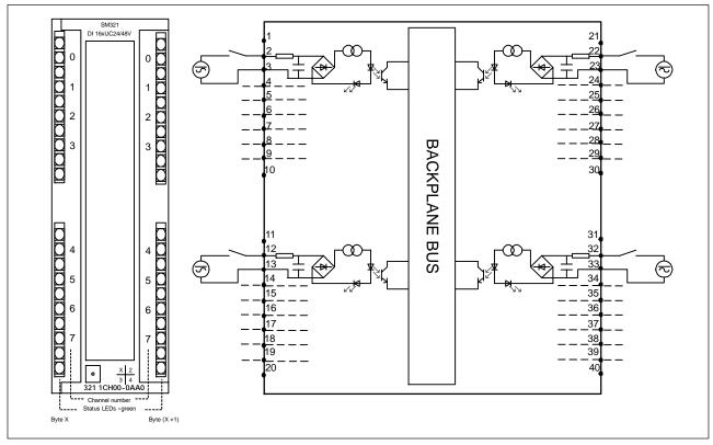
Figure 1 Connection Diagram of Digital Input Module SM 321; DI 16 x UC24/48 V
