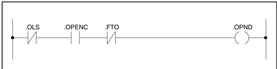
Figure A-34 VSS: OPND (EO) (N.O. FDBK) (IGNORE FDBK OVRD) (CLEAR CMMD ON FTO/FTC)
