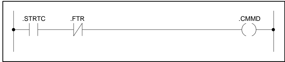
Figure A-151 MSS: CMMD (LATCH FTR)
