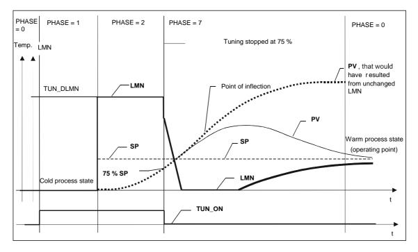
The schematic below illustrates the overshoot of the process variable when the excitation is too strong (process type III):
