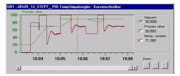
This screenshot shows the controller tuning when heating from ambient temperature 20°C to the operating point (70°C). Following this, a setpoint step change was controlled with a control zone. At the new operating point of 90°C, the controller was tuned again with negative manipulated variable excitation.
