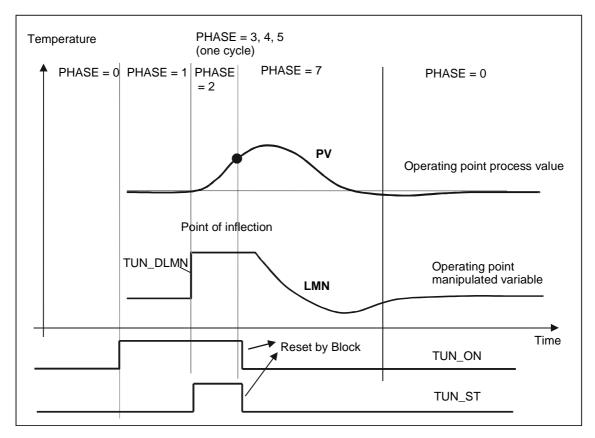
The schematic below illustrates the phases of tuning at the operating point started with TUN\_ST = TRUE:
