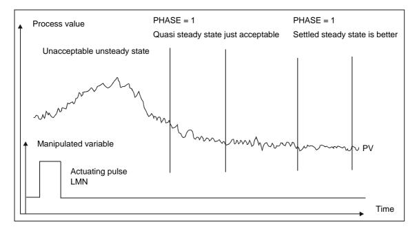
In Phase 1, the time prior to making the manipulated variable step change is used by FB 58 "TCONT\_CP" to calculate the process variable noise NOISE\_PV, the initial rise PVDT0 and the mean value of the manipulated variable (initial value of the manipulated variable LMN0).
