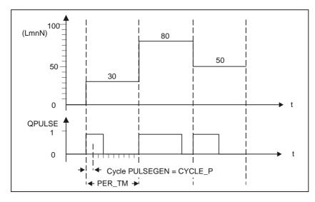
A manipulated variable value LmnN = 30 % and 10 PULSEGEN calls per PER\_TM therefore means the following:
