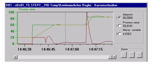
The screenshot above shows the controller tuning when heating from ambient temperature 20°C to the operating point (60°C). Following this, a setpoint step change from 60°C to 85°C is made within the control zone. The overshoot can be eliminated by reducing PFAC\_SP from 0.8 to 0.6.
