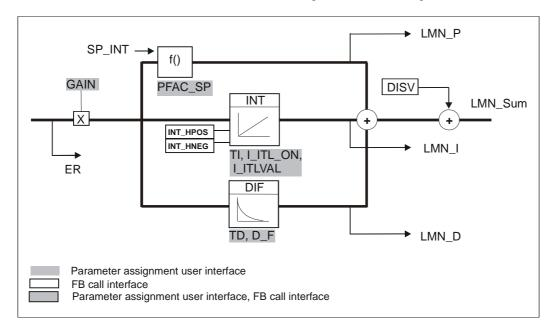
The schematic below is the block diagram of the PID algorithm:
