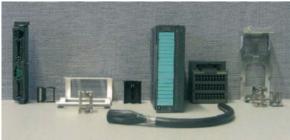
Figure 4-2 Components of the SM331 with the SIMATIC TOP connect system cables
