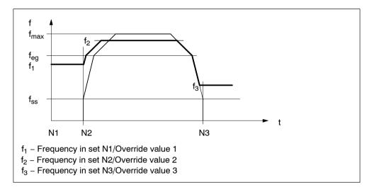
Fig. 9-8 Frequency profile with G64 or speed override
