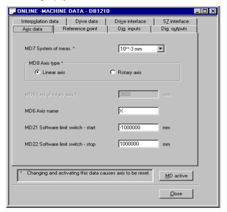
Fig. 5-4 Entering values for machine data
