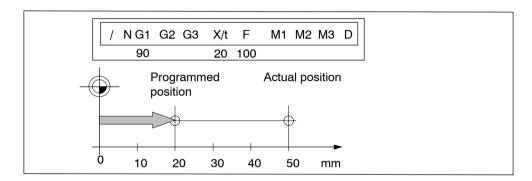
Fig. 10-1 Reference-measure input G90
