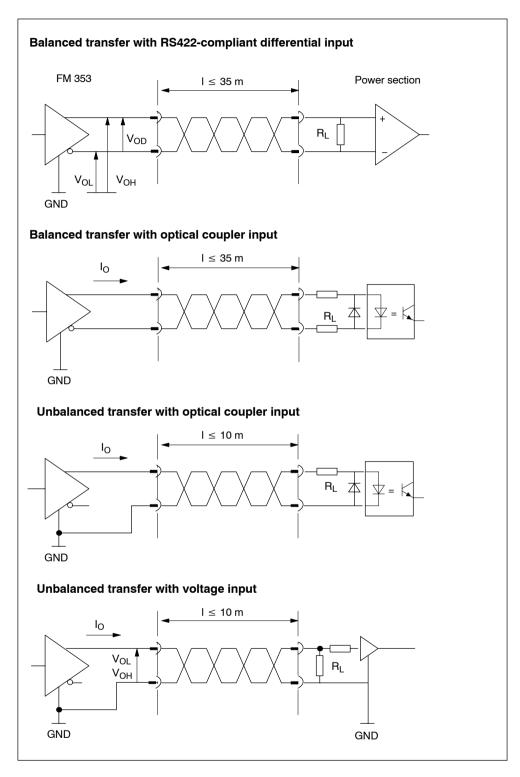
Fig. 4-3 Connection options for drive port output signals.
