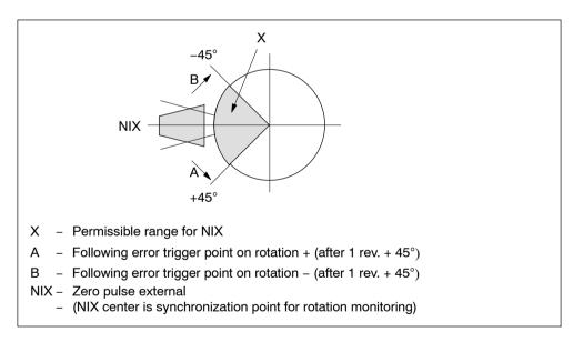
Fig. 9-10 Allowable range relative position for the external pulse
