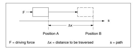
Fig. 2-1 Principle of a positioning action
