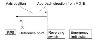
The value for the reference-point shift (MD27) is traveled after the synchronization point is reached.
