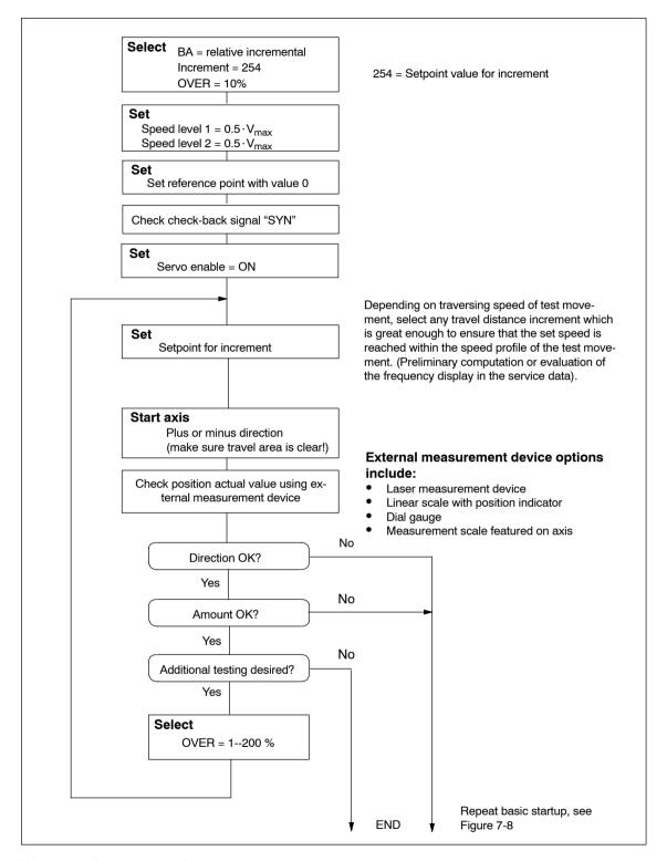
Fig. 7-9 Positioning verification
