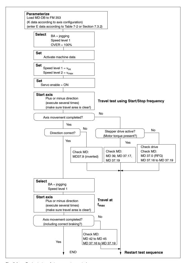
Fig. 7-8 Basic startup of stepper motor control
