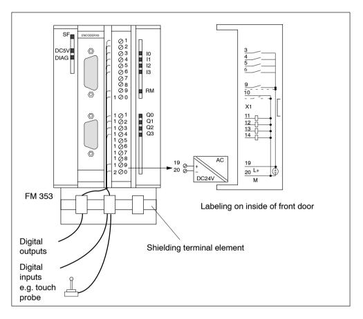
Fig. 4-9 Wiring of the front connector
