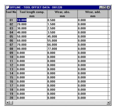
Fig. 5-7 Entering values for tool offset data
