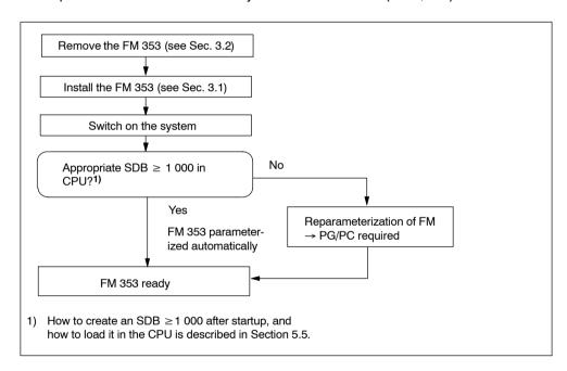
Fig. 3-1 Replacing the FM 353 with the system switched off
