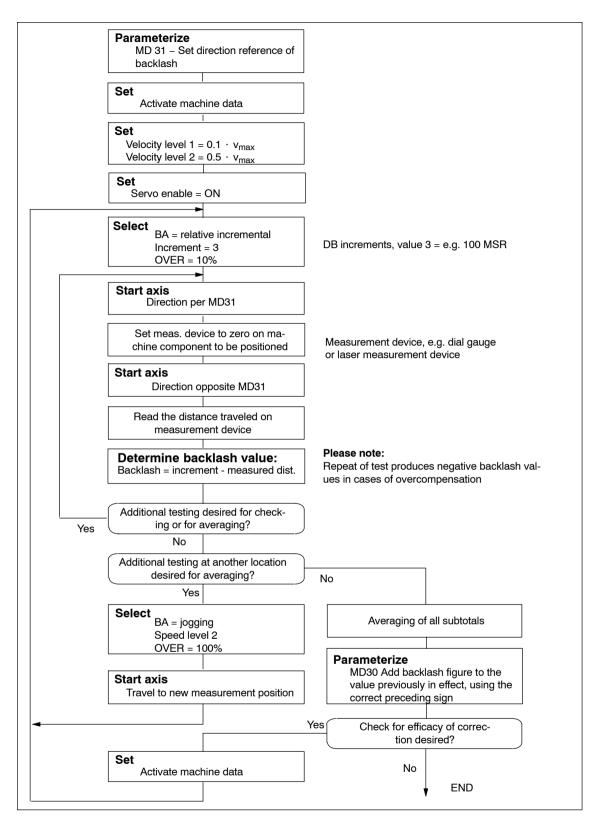
Fig. 7-12 Determining backlash and activating backlash compensation
