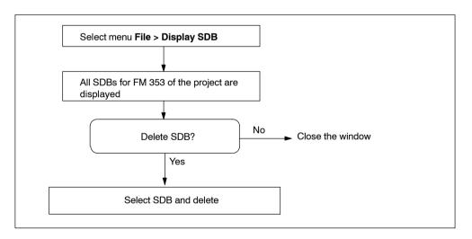
Fig. 5-10 Displaying/deleting SDB ≥ 1 000
