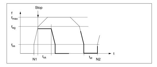
Fig. 9-9 Frequency profile for Stop or G60
