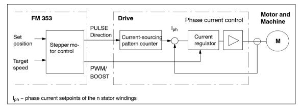
Fig. 7-10 Structure of the stepper motor axis
