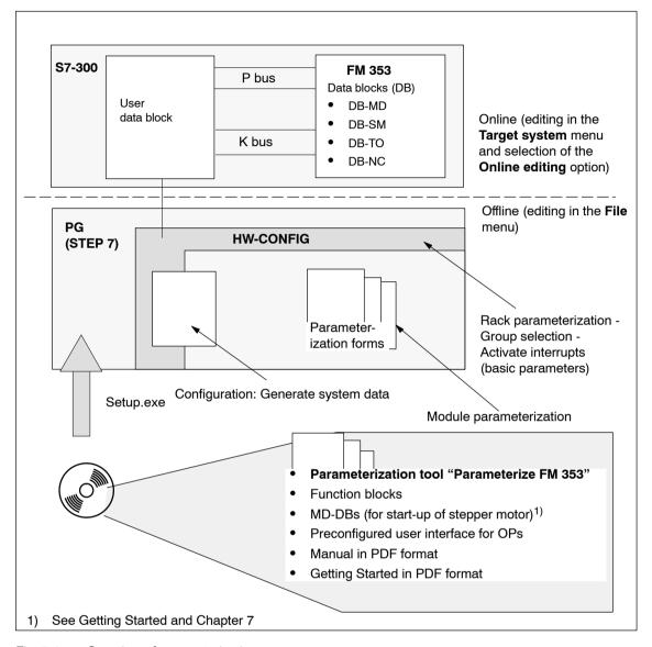
Fig. 5-1 Overview of parameterization
