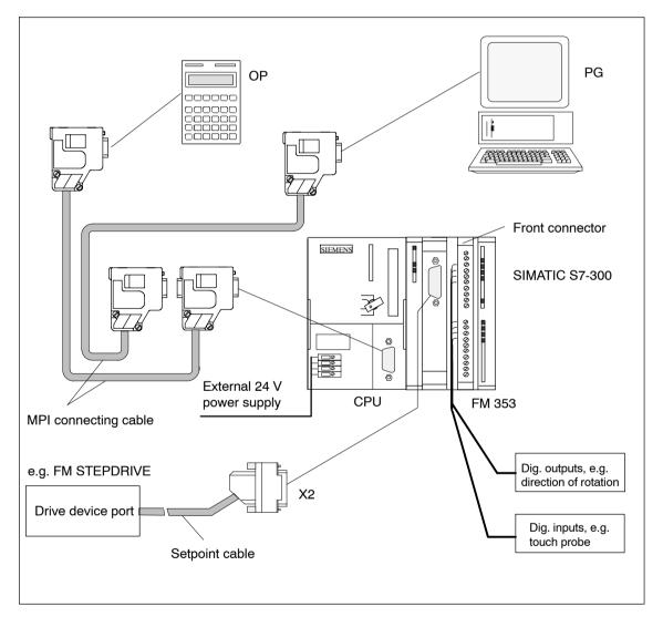
Fig. 4-1 Wiring an FM 353
