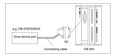
Fig. 4-5 Connecting a drive unit
