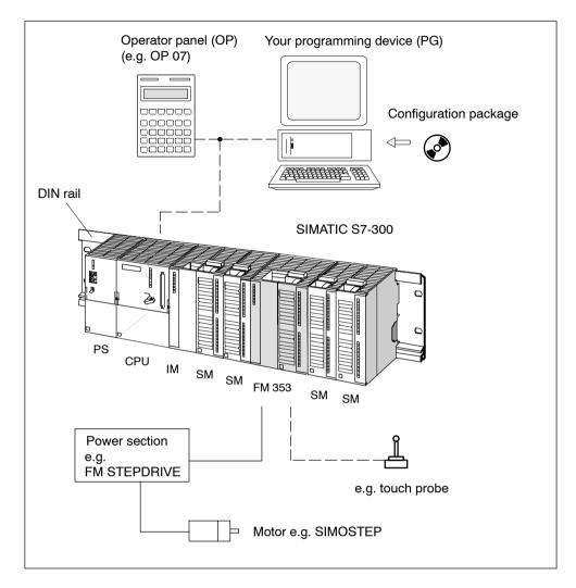
Fig. 1-2 System overview (schematic)
