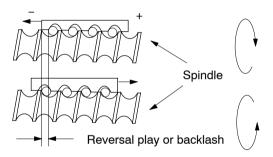
A backlash figure entered in the MD30 is calculated, with correction, by the stepper motor control as a factor of the current traversing direction of the axis. The result is an approximate compensation of backlash during positioning.
