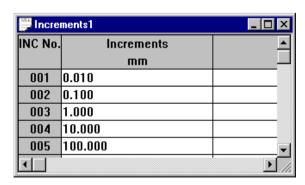
Fig. 5-6 Entering values for incremental dimensions
