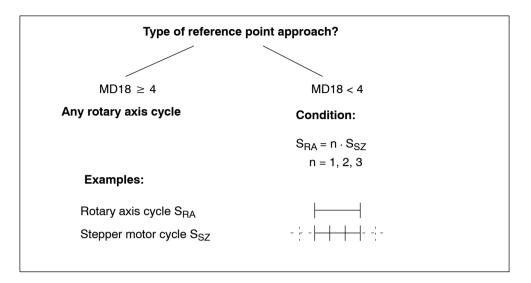
Fig. 9-5 Restriction for rotary axis cycle
