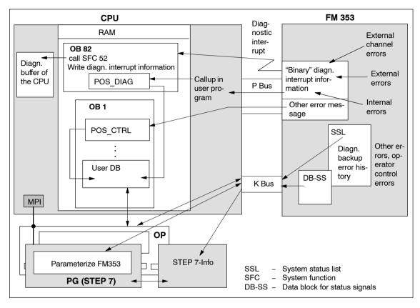
Fig. 11-1 Overview of diagnostics/errors
