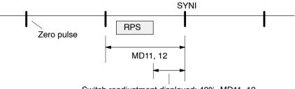
Switch readjustment displayed: 40% · MD11, 12 (suitable for high reducing speeds)
