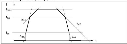
Fig. 9-7 Maximum speed frequency profile
