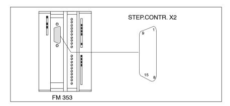
Fig. 4-2 Position of X2 connector
