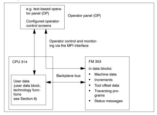
Fig. 8-1 Operator control and monitoring for the FM 353
