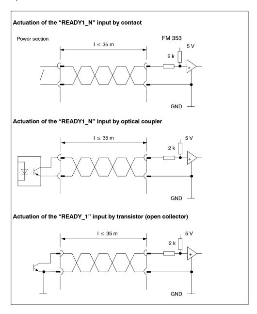
Fig. 4-4 Connection of the "READY1\_N" input
