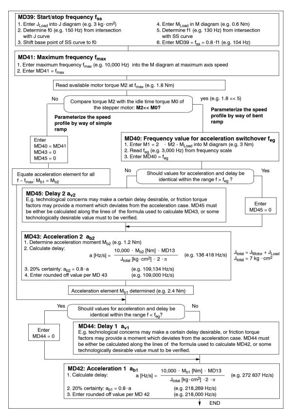
Fig. 7-7 Evaluation of operating characteristic curves
