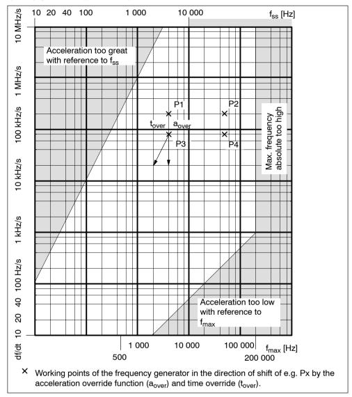
Fig. 5-5 Working range, frequency generator
