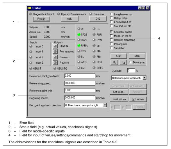
Fig. 7-2 Startup interface (e.g. for "Reference-point approach" mode)
