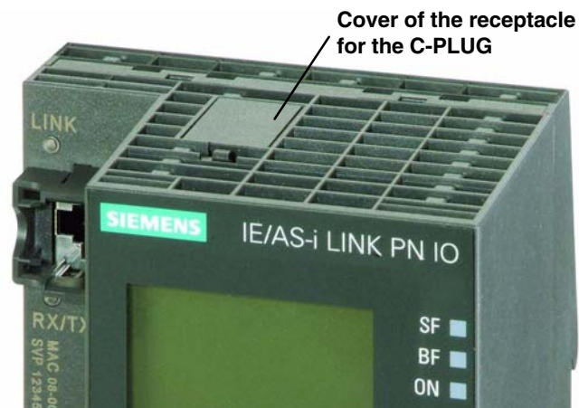
Figure 1-4 Position of the C-PLUG (removing the C-PLUG from the device with a screwdriver)
