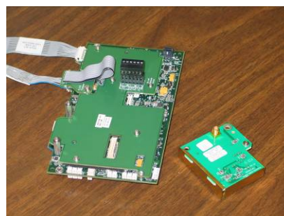
Flame Ionization DPM and Mezzanine
