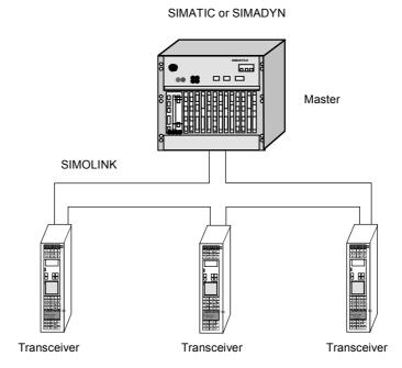
Fig. 8.3-13 Application example of master/slave functionality
