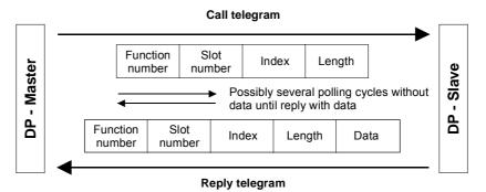
Fig. 8.2-5 Sequence of a Read and Write function
