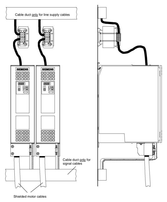
Fig. 3-19 Installation with separate cable ducts
