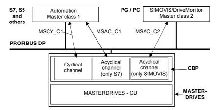
Fig. 8.2-3 Data-traffic channels of the CBP
