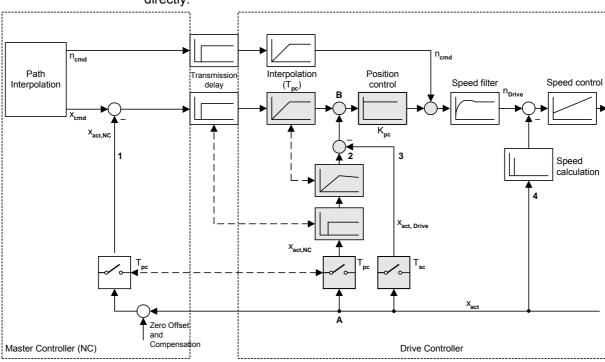
With DSC the actual position calculated inside the drive is also fed back directly:
