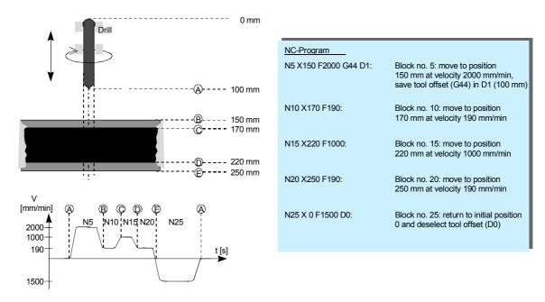
Fig. 9-5 Example of an Automatic Program
