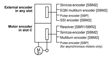
Fig. 9-10 Overview of Suitable Sensor Boards
