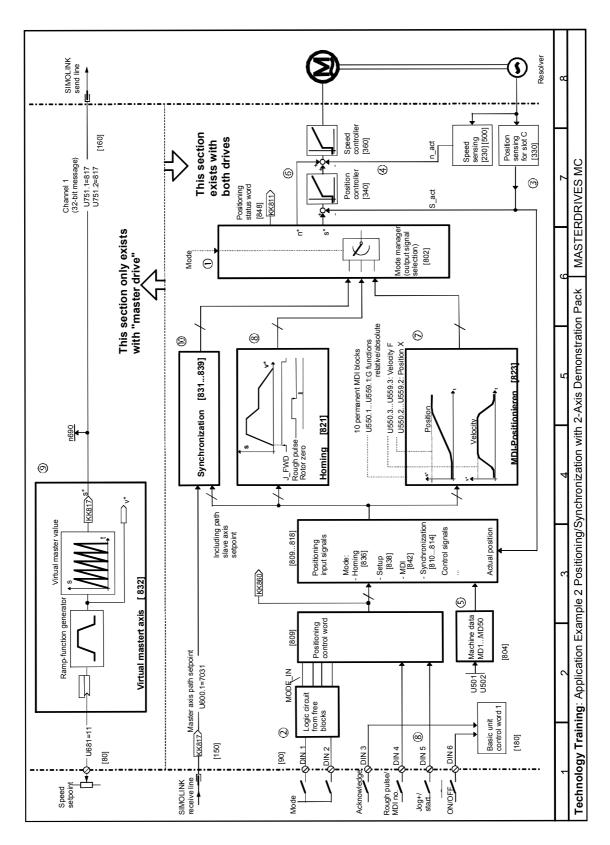
Fig. 9-45 Application Example 2: Positioning/Synchronization with 2-Axis Demonstration Pack
