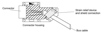
Fig. 8.4-8 Connecting the bus cables
