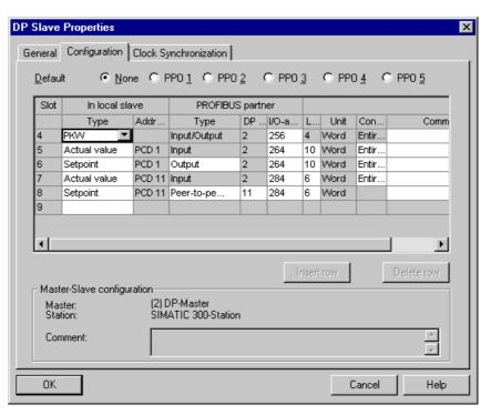
Fig. 9-49 Master axis CBP address 11
