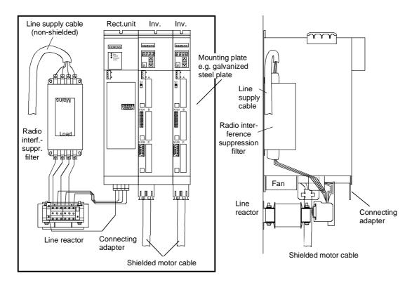
Fig. 3-14 Example of a Compact PLUS type unit with radio interference suppression filter and line reactor
