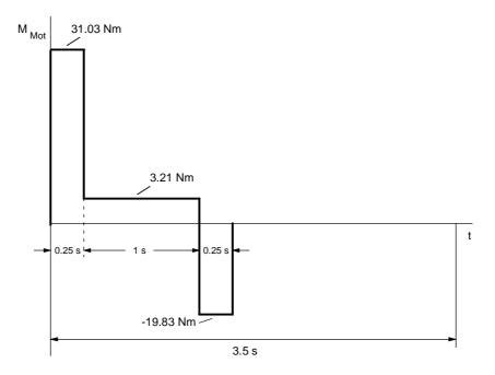
Fig. 11-15 Torque characteristic for forwards travel
