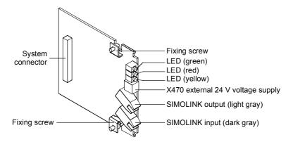
Fig. 8.3-6 SLB optional board (SIMOLINK board)
