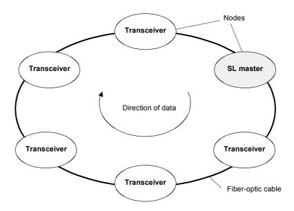
Fig. 8.3-12 SIMOLINK ring with SL master
