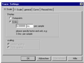
Display in data points: Scaling is performed in data points. The
