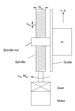
Fig. 11-6 Vertical spindle drive
