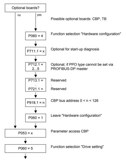
Fig. 8.2-18 Parameterization of "Hardware configuration" for Compact PLUS, CUMC and CUVC
