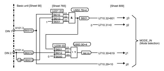
Fig. 9-46 Application Example 2: Circuit for Generating the Modes
