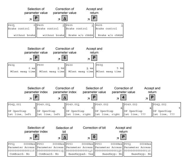
Some parameters may also be displayed without a parameter number, e.g. during quick parameterization or if "Fixed setting" is selected. In this case, parameterization is carried out via various sub-menus.
