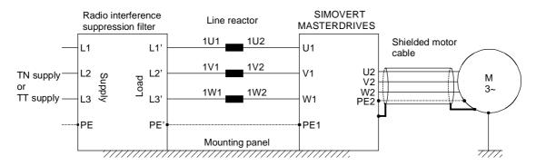
Fig. 3-4 Arrangement of the components
