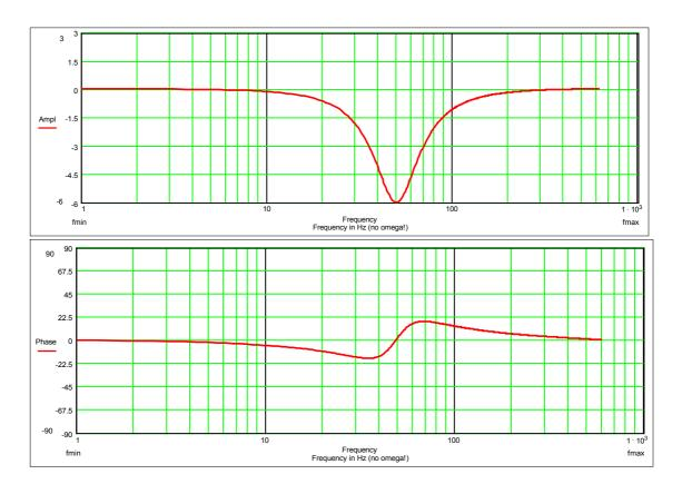
Example 3 Band-stop filter with full suppression and high quality: (P256 = 1; P254 = 50 Hz; P253 = 3.0; P257 = 0 %)
