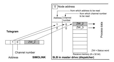
Fig. 8.3-8 Master drive 1, reading data
