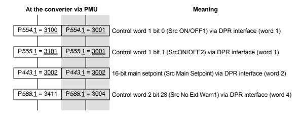
If the factory setting of the converter is used, the above example of parameterization is a functioning way of interconnecting process data (setpoints).
