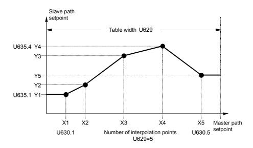
Fig. 9-40 Example of a cam with 5 interpolation points
