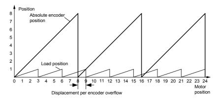
Example: Gear ratio 1:3, absolute encoder can count 8 revolutions
