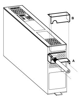
Fig. 3-17 Mounting the connecting adapter
