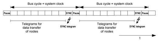
Fig. 8.3-2 SIMOLINK telegram traffic
