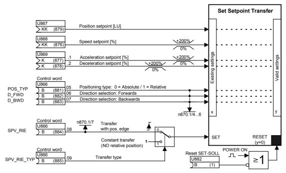
Fig. 7-3 Setpoint transfer input
