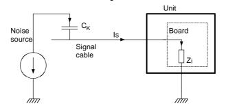
Fig. 3-5 Capacitive coupling for non-shielded signal cables
