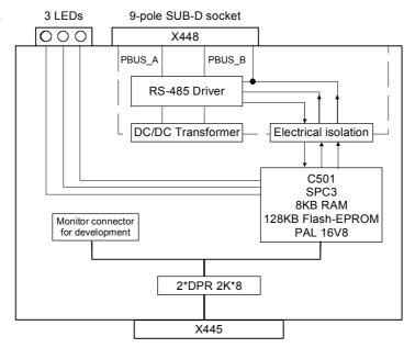
Fig. 8.2-40 Block diagram of the CBP
