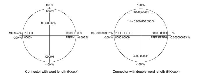
Fig. 4-3 Value range and assignment of the figure ranges for connectors
