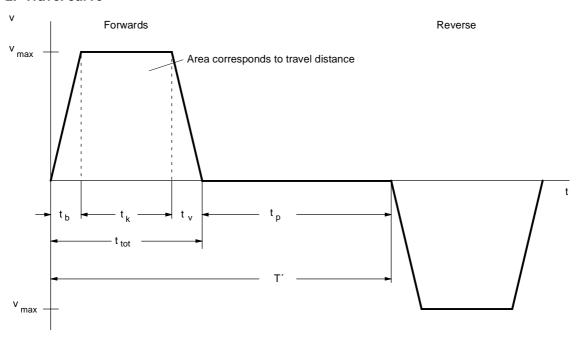
Fig. 11-13 Travel curve for forwards and reverse travel
