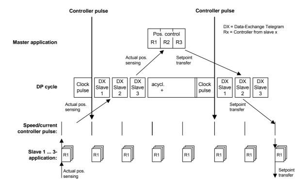
Fig. 8.2-31 Clock synchronous communication
