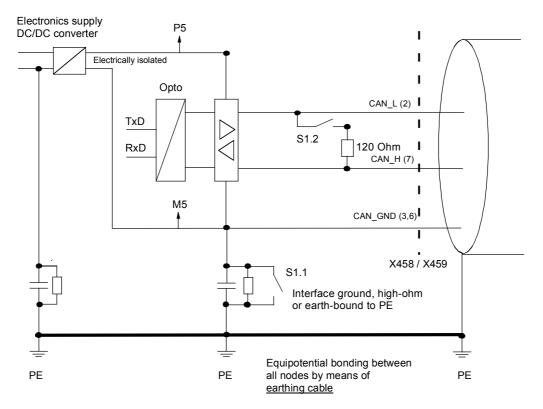
Fig. 8.4-12 Function of jumper strip S1
