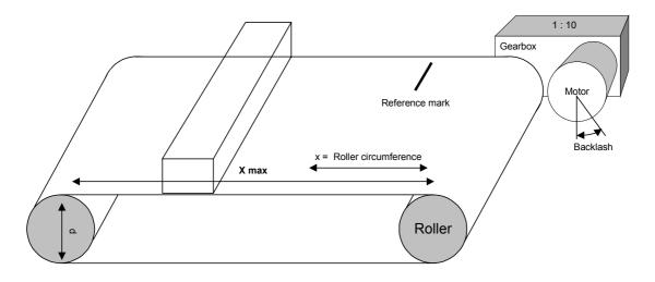
Fig. 7-7 Typical positioning application
