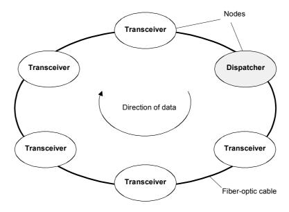
Fig. 8.3-3 SIMOLINK with dispatcher
