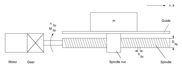
Fig. 11-5 Horizontal spindle drive
