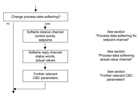
Fig. 8.4-18 Procedure for altering process data
