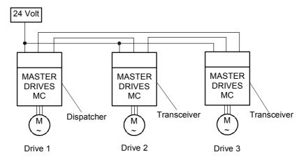
Fig. 8.3-7 Configuration example of peer-to-peer functionality
