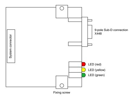
Fig. 8.2-1 View of the communications board
