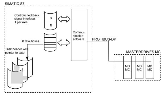
Fig. 9-42 Communication Interfaces from GMC-BASIC to Technology
