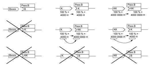
Fig. 4-9 Possible and impossible BICO connections
