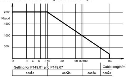
Possible baud rate depending on the cable length:
