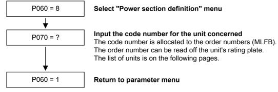
Fig. 6-3 Sequence for performing the power section definition
