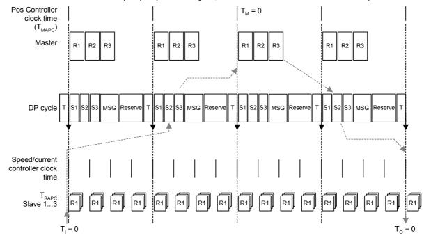
Fig. 8.2-37 Example: simplest DP cycle
