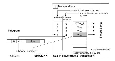
Fig. 8.3-10 Slave drive 2, reading data
