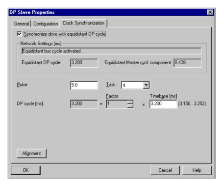
Fig. 9-53 Activation of the equidistance on the converter
