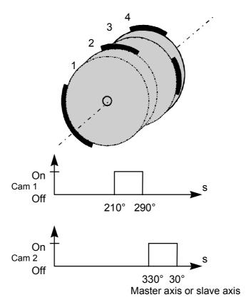
Fig. 9-9 Cam Controller with MASTERDRIVES MC
