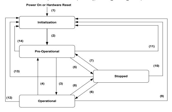
Fig. 8.5-1 State diagram of a device
