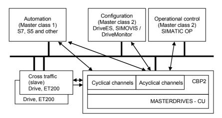
Fig. 8.2-4 Data-traffic channels of the CBP2
