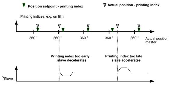
Fig. 9-8 Principle of Printing Index Synchronization
