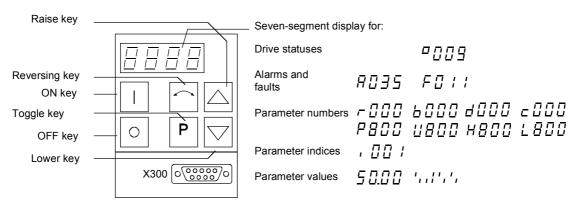
Fig. 5-3 PMU parameterizing unit
