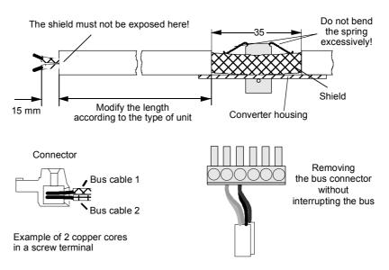
Fig. 8.1-9 Connecting up the bus cables
