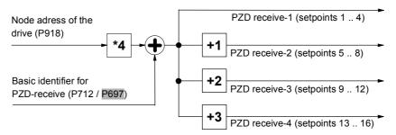
CAN identifier for the 1st PZD-receive CAN telegram (words 1 to 4): (value in 712 / P697) + (value in P918)\*4
