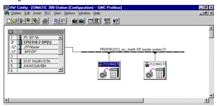
Fig. 9-48 Hardware configuration
