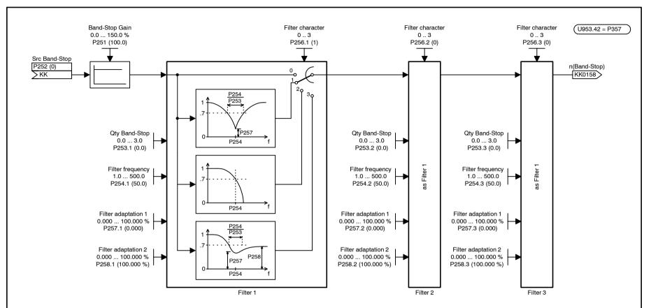
Please keep in mind that the resolution of the output variable diminishes as a smaller and smaller filter frequency (P254) is selected.
