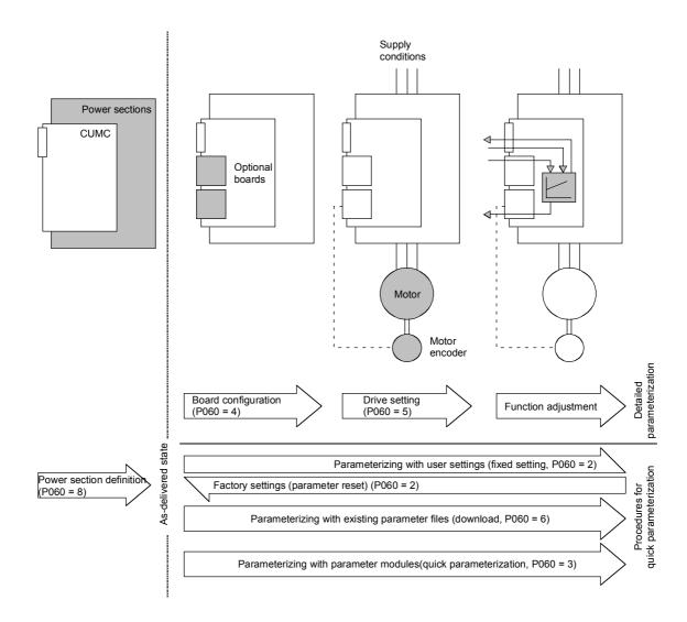
Fig. 6-1 Detailed and quick parameterization
