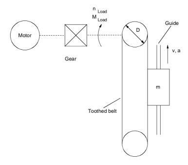
Fig. 11-3 Lifting drive
