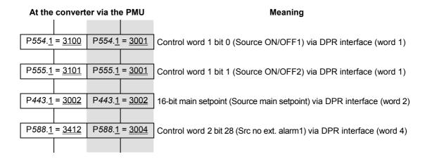
Based on the factory setting of the converter, the above example of parameterization represents a functioning method of connecting (softwiring) the process data (setpoints).
