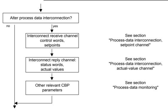
Fig. 8.2-20 Procedure for changing process data
