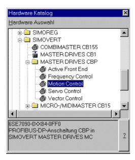
The type of PPO is selected in the hardware manager from the register "Configuration" of the "Characteristics – DP slave" mask which is automatically shown on the screen when the selection (e.g. Motion Control) is confirmed.
