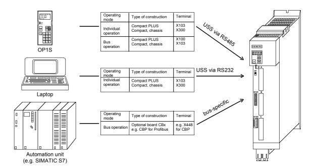
Fig. 6-5 Parameter transfer from various sources by download
