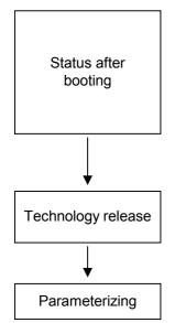
If the parameter structure between the firmware status before booting and the new firmware has not changed, then the units retain the same operating status (e.g. °009 ready for operation) and the parameterization (see below) as before.
