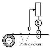
If the printing index comes too late, short-time acceleration has to take place to make up the position delay again. Beforehand, the position setpoint and actual value are set in the counter-direction in order to create the correct reference to the mechanical system.
