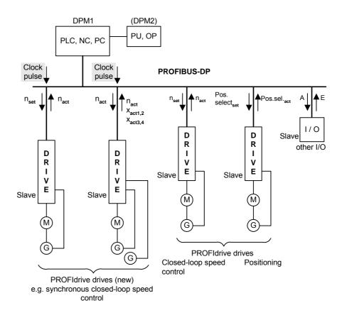
Fig. 8.2-30 Clock synchronous monomaster operation (DPM1)
