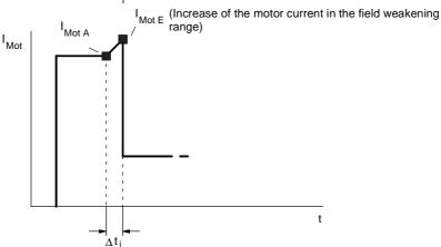
Fig. 11-10 Example of motor speed and motor current in a time segment  $\Delta t_i$
