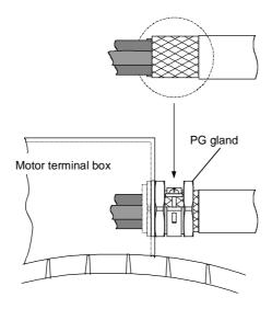
Fig. 3-11 Shield connection at the motor
