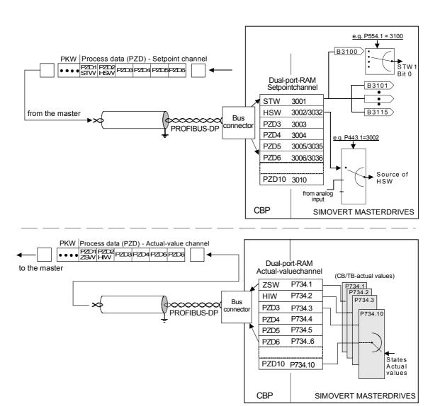
Fig. 8.2-21 Example of process data interconnection of the first CB board in function classes Motion Control Compact PLUS, CUMC and CUVC
