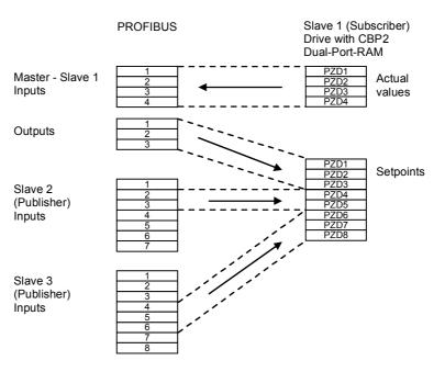
Fig. 8.2-25 Example of a cross-traffic configuration
