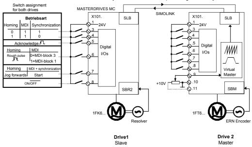
Fig. 9-44 Application Example 2: Hardware Configuration and Wiring
