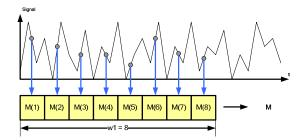
**Note** Window length "w1" is valid for the fine range while window length "w2" is used for the coarse range. For a correct analysis of the hydraulic axis, the fine range has to be set in a way that only small changes of measurement signals take place in this range. Thus, the window length can be better adjusted to the measurement signals to be expected.
