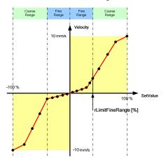
**Note** For setting the "rLimitFineRange" parameter, the percentage value of the actuating variable for which a significant movement of the hydraulic axis is detectable can be empirically determined via the JOG function of the technology template.
