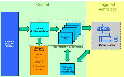
The technology object controlled by the FB 520 "GetCharacteristics" block is not allowed to be controlled by another part of the application program while FB 520 "GetCharacteristics" is active.
