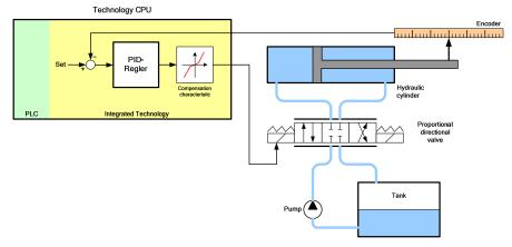
Generally, a hydraulic axis consists of a hydraulic cylinder, which is controlled via a proportional directional valve. The valve controls the flow/pressure of the hydraulic oil in the cylinder, which is provided via the pump. The valve is activated via the control output of the technology CPU.
