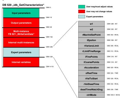
Figure 6-2 Structure of the instance data block
