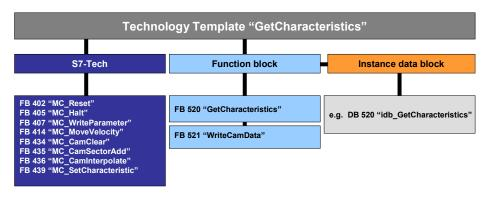
**FB 520 "GetCharacteristics"** contains the complete functionality for determining the compensation characteristic of a hydraulic axis. To do this, the function block performs measurements at the hydraulic axis in order to determine the compensation characteristic and saves this measured value in the instance data block of FB 520.
