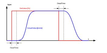
Figure 3-3 Dead time between the setpoint output and the movement of the hydraulic axis
