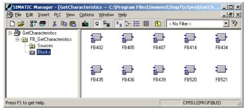
Figure 5-1 Blocks of the technology template
