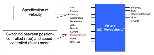
Figure 9-1 Selection of open-loop mode via FB 414 "MC\_MoveVelocity"
