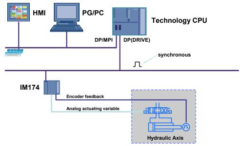
Figure 2-2 Typical structure for controlling a hydraulic axis
