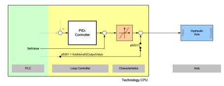
**Note** The shown procedure of switching between speed control and position control could be used as background information. With the technology template you could manage the switching with mode 6 and mode 7 of the function block.
