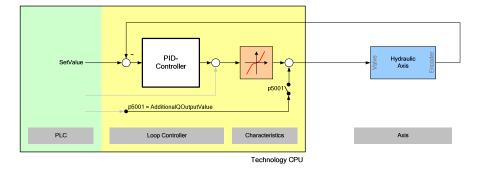
Via compensation characteristic, the linear behavior of the controller is, in the technology CPU, adapted to the non-linear behavior of the hydraulic axis.
