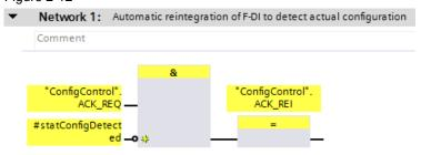
Program the selection of configurations. To ensure that the selection is selected only once after the CPU is started and does not change even if the wiring is changed during operation, evaluate the static variable "statConfigDetected".
