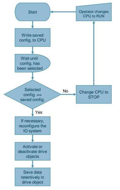
Figure 3-4: Possible sequence for configuration control in central structure
