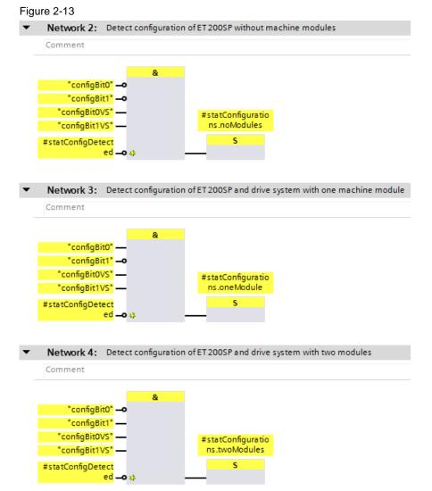
**Note** When selecting the configuration, note that substitute values are used for the inputs of the F peripherals in certain situations, e.g. when starting the F system or in the event of F periphery/channel errors.
