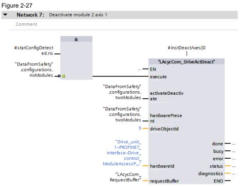
4. To activate or deactivate the motor module depending on the actual configuration, create the variable of the configuration in which the motor module exists at the inputs "activateDeactivate" and "hardwarePresent".
