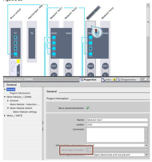
Apply the HW identification of the Control Unit to the "hardwareld" input. These can be found in the properties of the control unit or in the system constants. Figure 2-29
