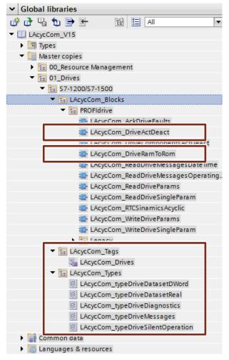
2. Drag the FB "LAcycCom\_DriveActDeact" to activate or deactivate a drive object in the next network and create an instance.
