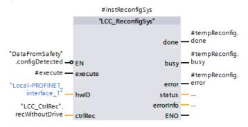
4. Call the FB "LCC\_ReconfigureSys" in the next network again and interconnect it in a manner that it reconfigures the IO system if a configuration with the drive system was selected. You may use the same instance for this but must ensure that only one call is processed per cycle.
