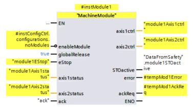
Figure 3-3: Calling the FB "MachineModule" for machine module 1
