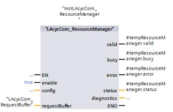
The default configuration is sufficient for this application. The input "config" is therefore not connected.
