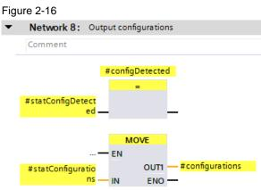
10. Open the FB "Main\_Safety" and call the newly created FB in it. Connect the outputs with a standard DB to transfer the configuration selection to the standard user program.
