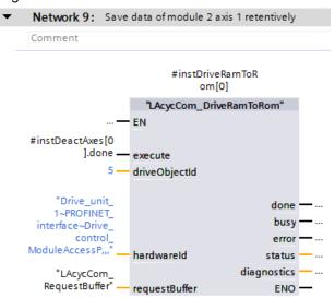
9. Repeat steps 2 to 8 for each additional optional motor module. Use a separate instance for each.
