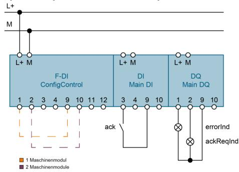
Figure 2-32: Wiring ET 200SP station with minimum configuration
