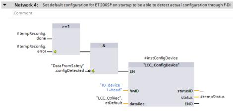
7. Program the configuration control of the remaining configurations of the ET 200SP station. You may use the same instance but must ensure that a maximum of one call is processed per cycle.
