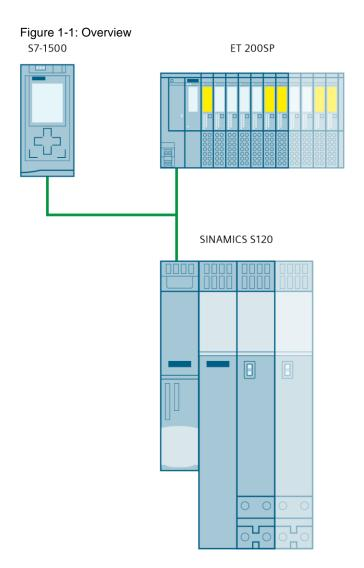
The actual configuration can, for example, be selected in a fail-safe data block. Since data cannot be remanently stored in error-proof data blocks, you must define the selection using start values and thus adapt the data block for different projects. This application example shows you how you can select the actual configuration via the wiring of an F-DI module instead and thus do not have to adapt the user program and also do not require an engineering system during commissioning.
