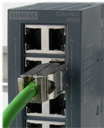
Figure 6-2 Plugging in the IE FC RJ45 Plug 180
