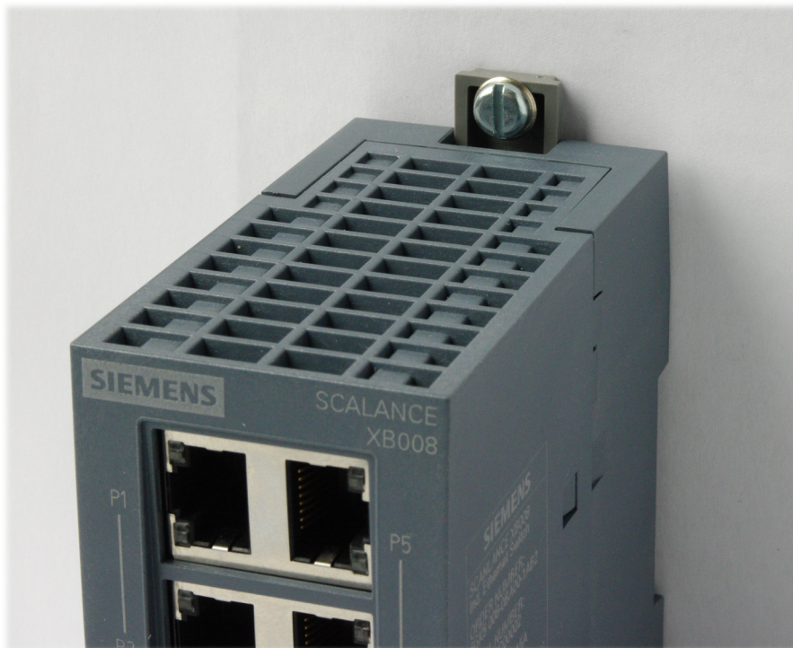
Figure 5-5 Wall mounting of the SCALANCE XB-000
