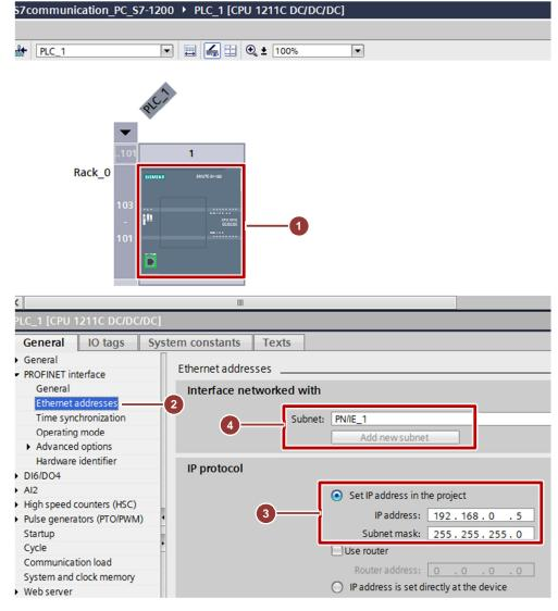
The connection between the subnet, PN/IE\_1, for example, and the S7-1200 is now displayed in the "Network View" of the Devices and Networks editor. Figure 3-7
