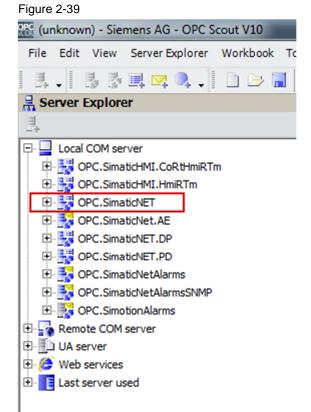
The configured S7 connection named "S7\_Connection\_1" is displayed in the Server Explorer under OPC.SimaticNET in the "\S7:" folder.
