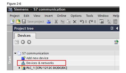
In the Network View or Device View of the devices and networks editor you click the PROFINET interface of the S7-1200 CPU.
