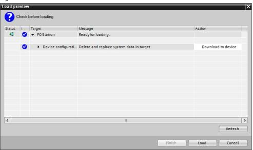
Commissioning of the PC station is completed after downloading of the configuration.
