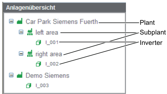
Figure 3-3 Example: Tree structure in the Plant overview
