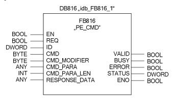
With this FB 816 you transmit PROFlenergy commands to a PROFlenergy capable device. The input data is stored in the "CMD\_PARA" data area addressed by the ANY pointer . The output data is stored in the RESPONSE\_DATA data area addressed by ANY pointer.
