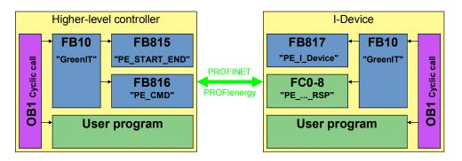
The FB10 "GreenIT" function block summarizes the actual PROFlenergy block calls and provides a comfortable interface through its instance data block for the HMI.
